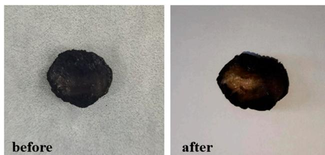
**Figure 11.** Photos of PNIPAm/PPy before and after material desorption (20 times; thickness of 2 mm).
