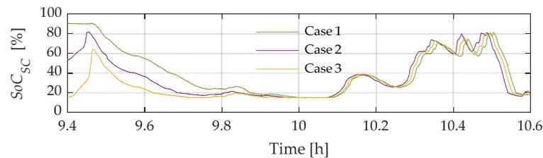
**Figure 15.** Response of SC-ESS to the LP filter under its three  $SoC_{SC}$  conditions: Case 1 with  $SoC_{SC}$  around 90%. Case 2 with  $SoC_{SC}$  around 50%, and Case 3 with  $SoC_{SC}$  lower than 20%.
