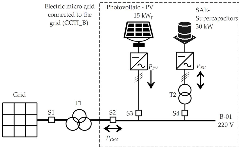
Figure 7. Grid-connected microgrid at the Micro-Grid laboratory (CCTI-B).
