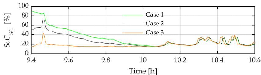
**Figure 19.** Response of SC-ESS to the MA filter in its three  $SoC_{SC}$  conditions: Case 1, greater than around 90%, Case 2, around 50%, and Case 3, less than 20%.
