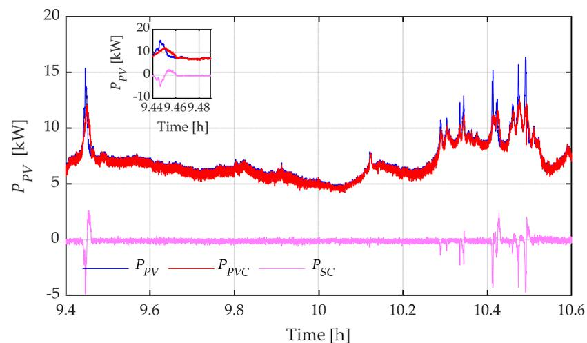
**Figure 22.** Results of the response of SC-ESS (case 3) to fluctuations in the input PV power  $P_{PV}$  with the RR filter and its compensated PV power response  $P_{PVC}$ .
