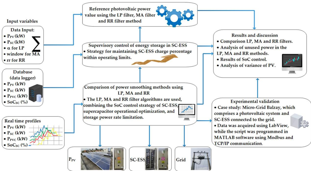
Figure 1. Representative scheme of the proposed methodology.
