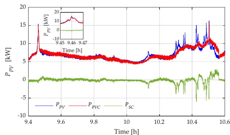
**Figure 12.** Results of the response of SC-ESS (Case 1) to input PV solar power fluctuations  $P_{PV}$  with the LP filter and its compensated PV solar power response  $P_{PVC}$ .
