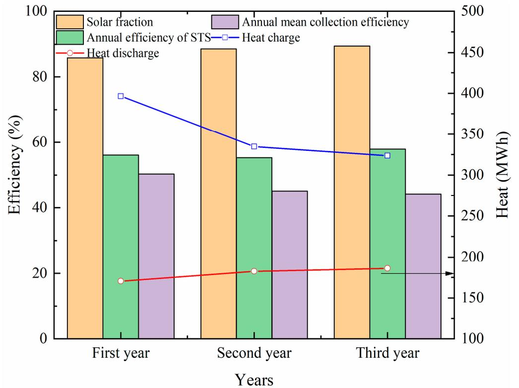
Figure 18. System performance change over three continuous years.
