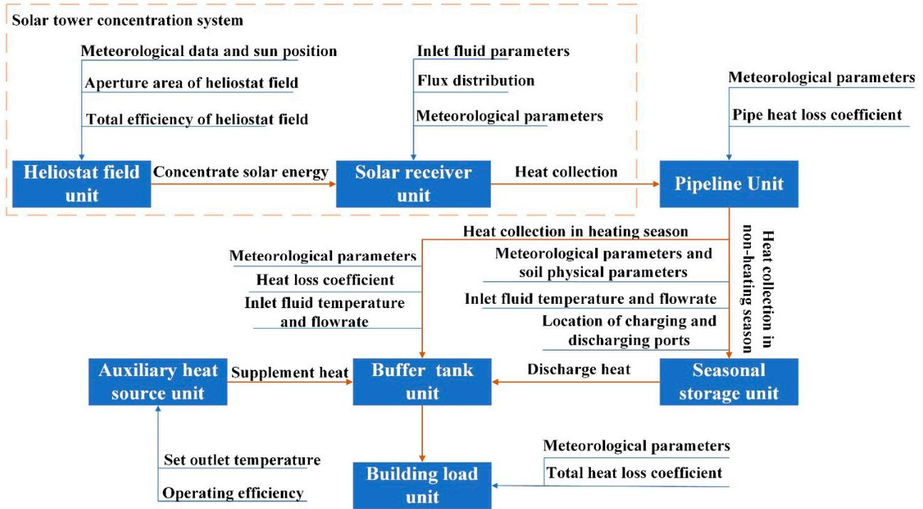
Figure 5. Transfer relationship of energy flow of core components.
