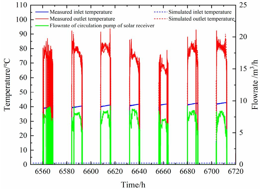
Figure 7. Simulated and measured inlet and outlet temperatures of solar-tower concentration system.
