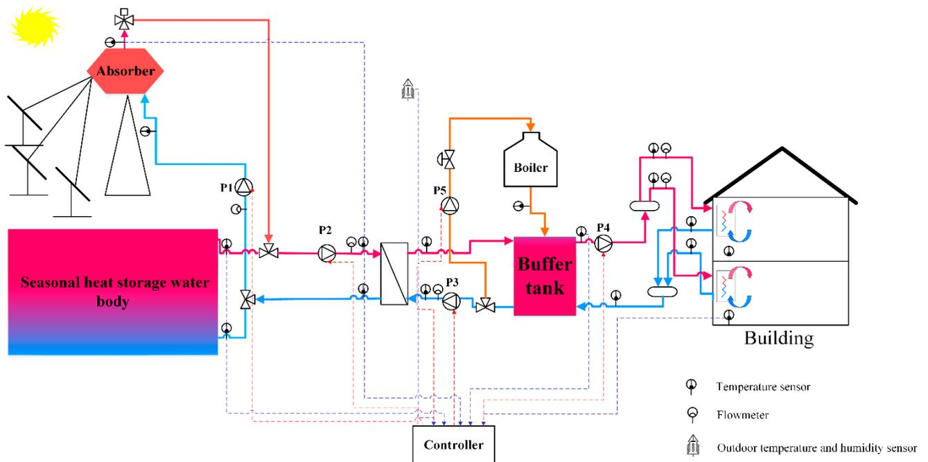
Figure 3. Schematic of solar-heating system. (The dashed lines represent the signal flow, while the solid lines represent the heat and mass flow).
