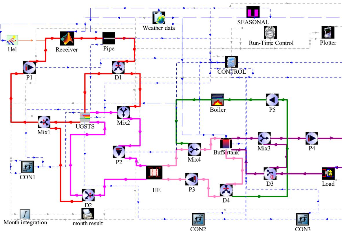
**Figure 6.** TRNSYS simulation platform for the solar-heating system. (The dashed lines represent the signal flow, while the solid lines represent the heat and mass flow).
