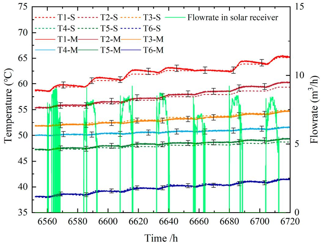
Figure 8. Experimental and simulation values of temperature at different heights in STS (S: simulation; M: measured).
