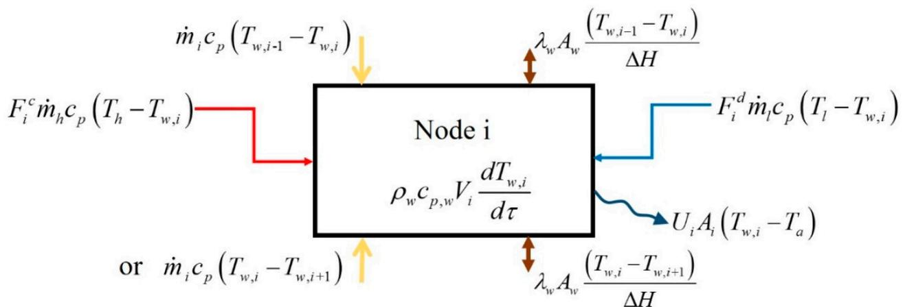
Figure 4. Energy transfer at node of buffer tank.
