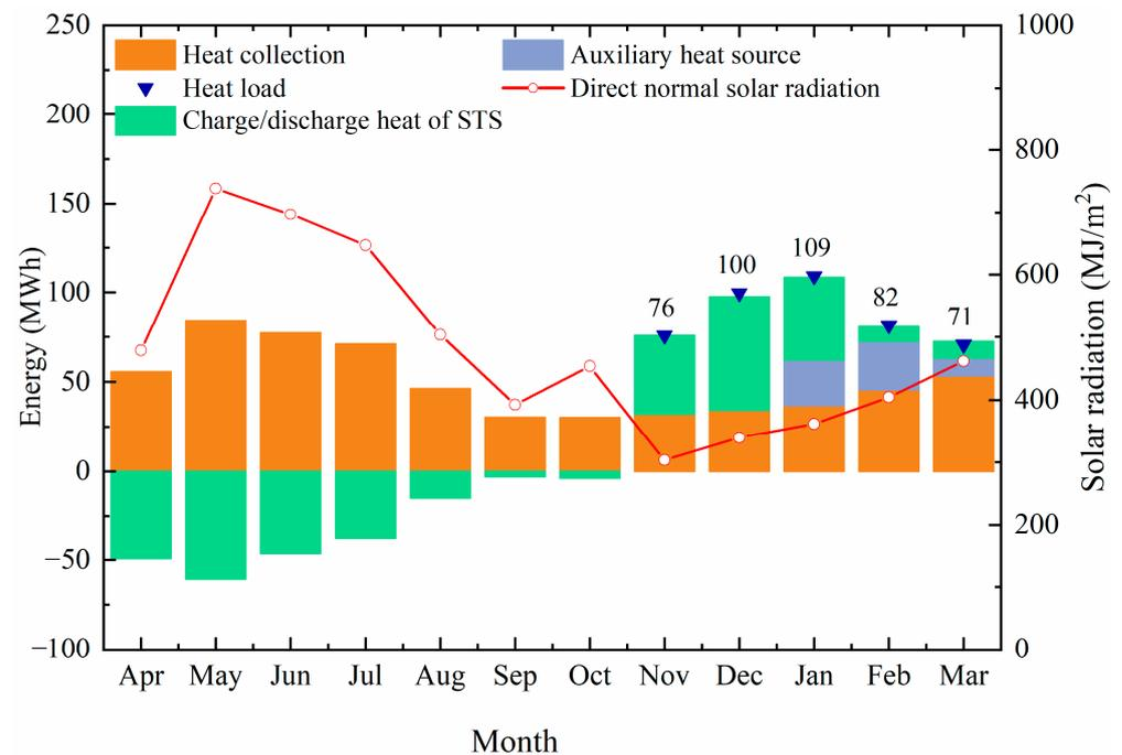
**Figure 16.** Operation energy flow in the first year.
