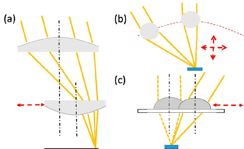
**Figure 4.** Sunlight tracking performed by the concentrator optics of the tracking-integrated system. (a) Lateral displacement of two plano-convex lenses. (b) Spherical GRIN lenses with two-directional displacement. (c) LC as a concentrator element with electrode-activated displacement.
