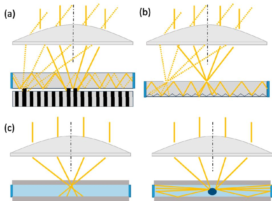
**Figure 8.** Self-tracking systems using solid waveguides by means of the phase changes of materials (a) or switchable transparency properties (b), and using liquid waveguides (c).
