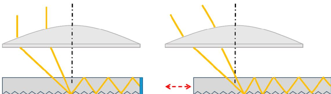
**Figure 7.** Lateral displacement of the waveguide when the AOI is different from the normal angle.
