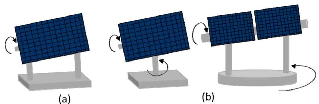
Figure 3. Some designs of solar trackers: (a) single-axis, and (b) two-axis pedestal-mount (left) and carousel (right) [9].
