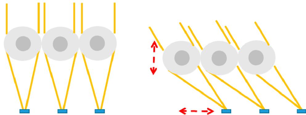
**Figure 9.** Two-state tracking system; the primary optics describes a first vertical movement. After radiation concentration, the solar cell array moves laterally to follow the displacement of the focal point.
