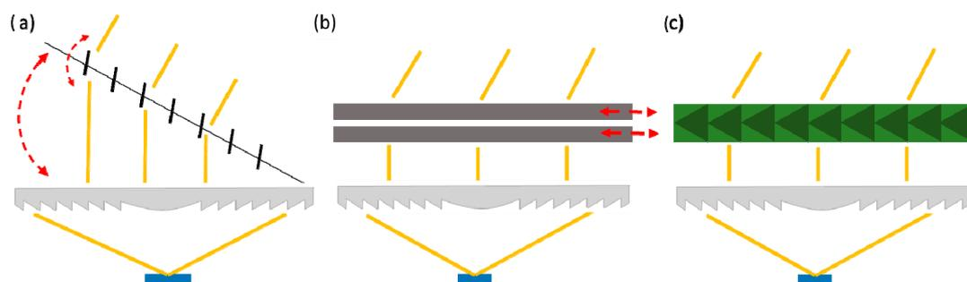
**Figure 5.** Scheme of different systems with external tracking to the CPV module (beam steering). It shows the representation of the basic CPV system with the addition of mirror rotation and elevation of the micro-heliostat array (a), lateral displacement of the second lens array (b), and prism-shaped liquid crystals with a different refractive index (c).
