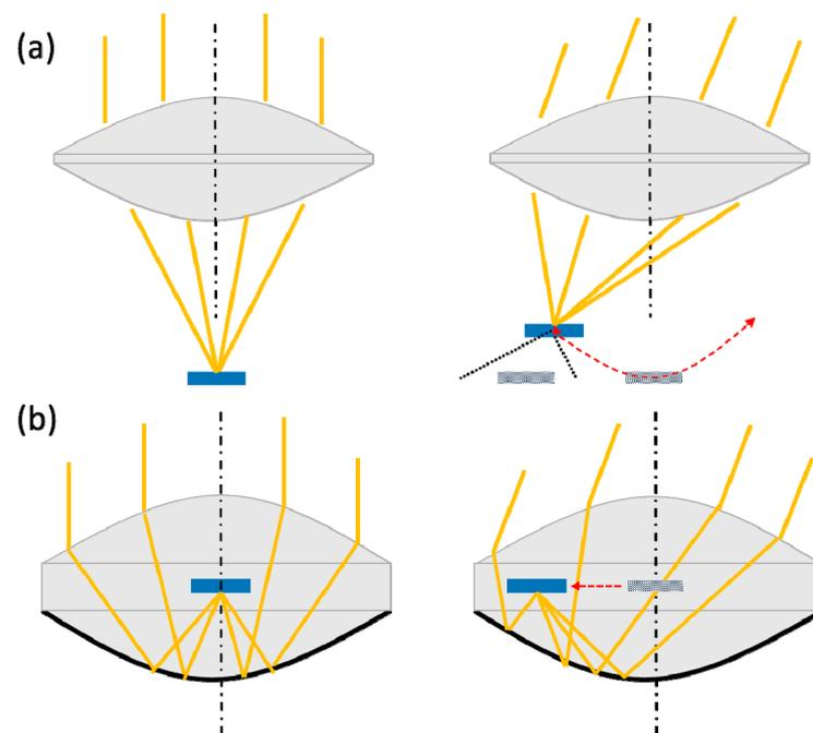
**Figure 6.** Diagram of the integrated tracking systems with mobile solar cells. (a) Focusing system using aspherical bi-convex lenses. The dashed line describes the movement in two directions (Petzval curvature) made by the focal point of the lens. (b) Focusing system with sandwich configuration to achieve only a lateral displacement of the receiver.
