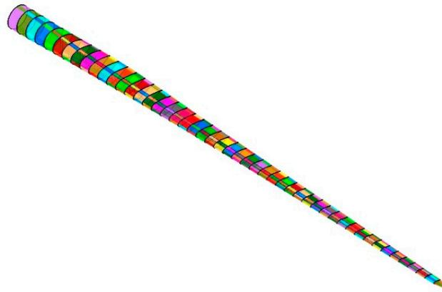
**Figure 5.** Blade model established by NuMAD.
