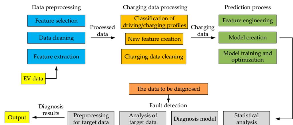
Figure 4. Framework of the proposed data-driven battery charging capacity diagnosis method.
