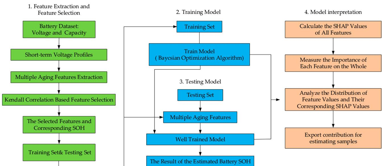
**Figure 3.** The framework of the battery SOH estimation based on the interpretable stacking ensemble model with the Bayesian optimization algorithm.
