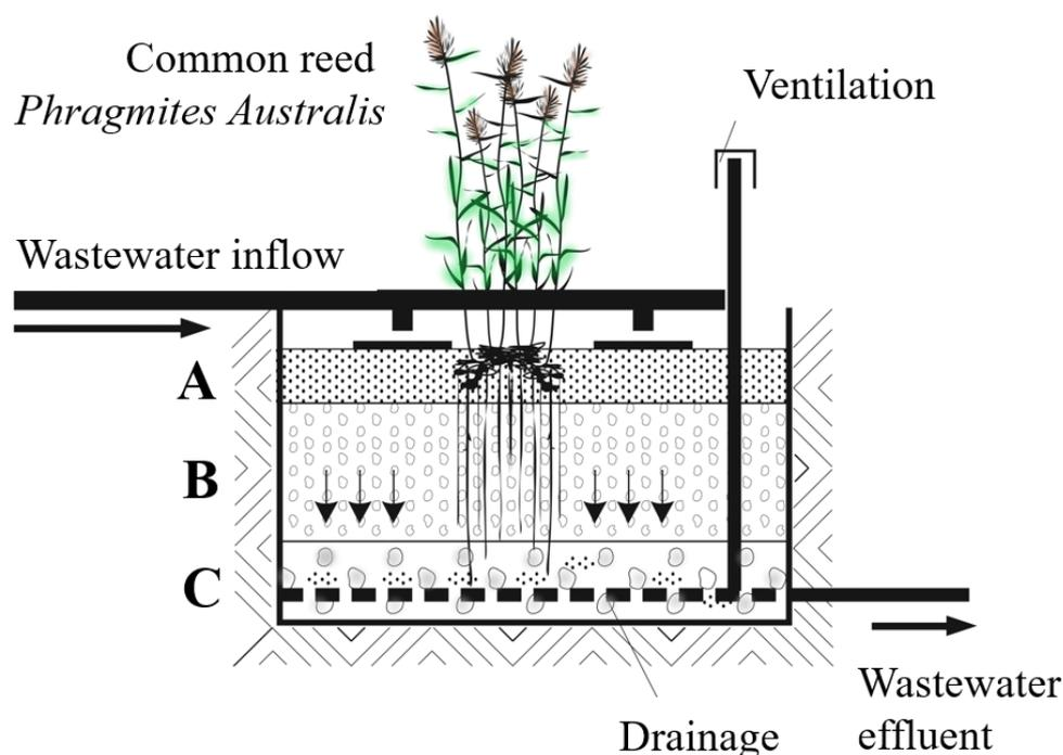
**Figure 1.** Cross-section of a vertical flow constructed wetland bed (layer: A—0.15 m, B—0.40 m and C—0.15 m).
