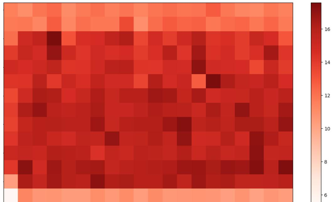
**Figure 2.** Power measurement matrix of an LED light bulb, measured using the TEST\_ORIG profile. Each cell represents the AC power consumed by the load in a single AC period during the measurement. The matrix is filled in a row-major way during the measurement. The size of the measurement matrix is determined by  $r$  and  $h$ .
