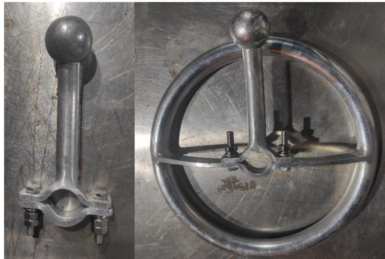
**Figure 8.** Ring parallel gap of insulator.
