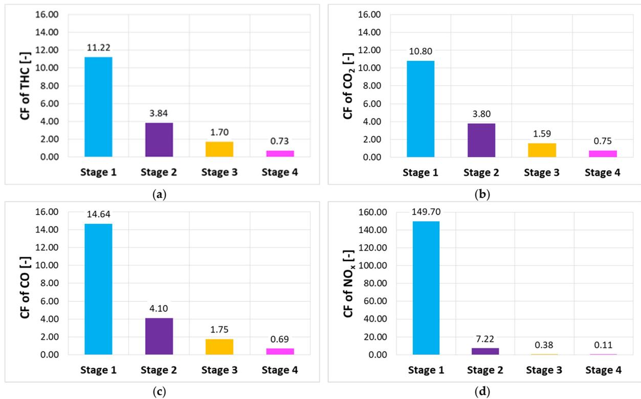
Figure 11. Road emission share coefficients in individual stages of the test for (a) THC, (b) CO<sub>2</sub>, (c) CO, and (d) NO<sub>x</sub>.
