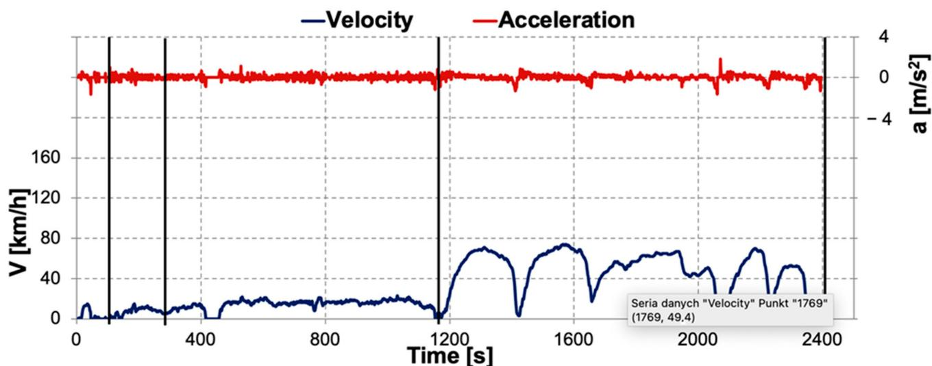
Figure 5. Vehicle velocity profile. (Vertical lines mark the end of the subsequent stages of the study).
