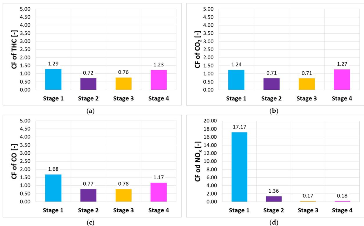
Figure 12. Specific emission share coefficients in individual stages of the test for (a) THC, (b) CO<sub>2</sub>, (c) CO, and (d) NO<sub>x</sub>.
