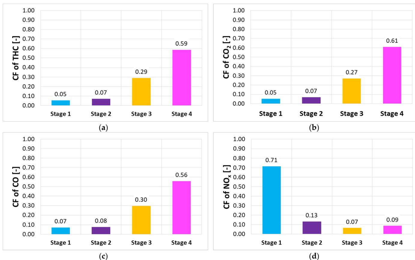
**Figure 10.** Coefficients of mass share of the emission components in individual stages of the test (a) THC, (b) CO<sub>2</sub>, (c) CO, and (d) NO<sub>x</sub>.
