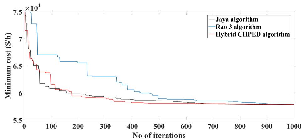
**Figure 4.** Minimum price convergence curve for case 1 of test system 2.
