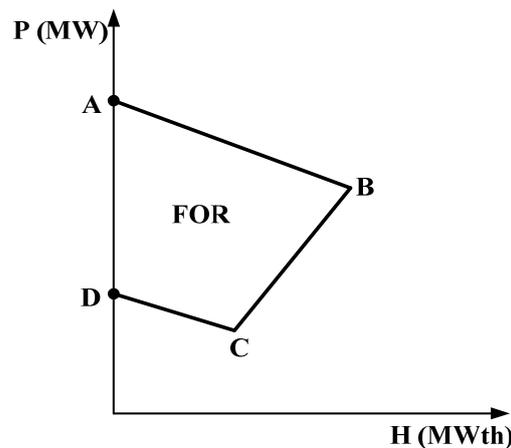
Figure 1. FOR of a CHP unit.
