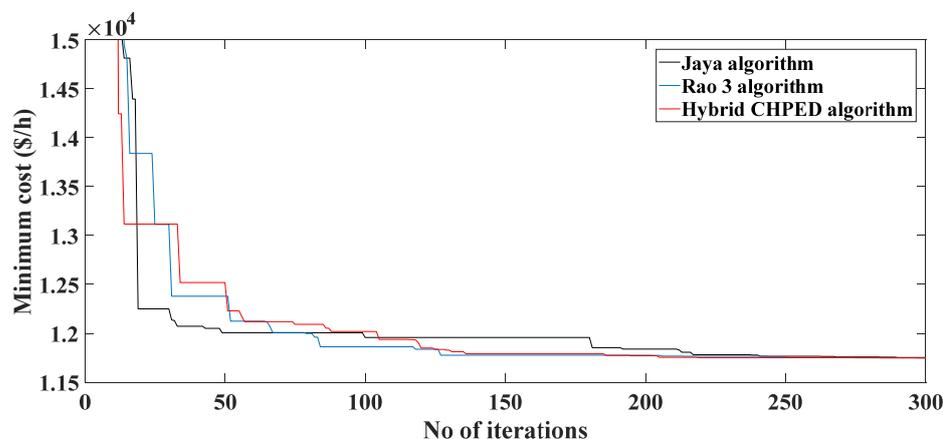
**Figure 3.** Minimum price convergence curve for the 5-unit test system.
