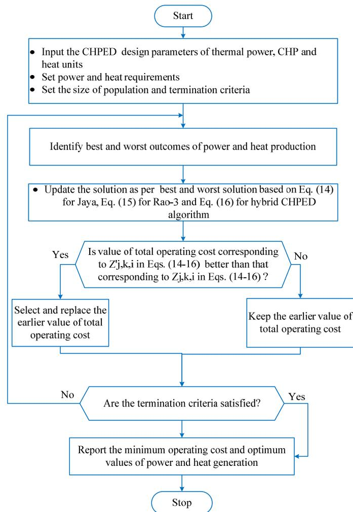
Figure 2. Flow chart of the proposed CHPED algorithm.
