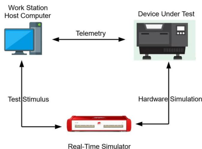
**Figure 2.** Implementation of the digital twin using hardware in the loop system [7]. Applying unified testing both virtually and physically on the same unit provides faster error tracking and an easier understanding of the process.
