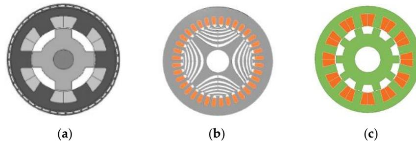
**Figure 5.** Cross-section of different motor cores: (a) induction; (b) synchronous reluctance; (c) switched reluctance [39,47].
