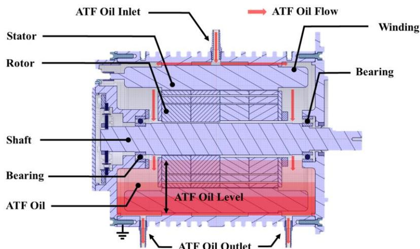
Figure 10. Flow channel for oil spray cooling method by [78].
