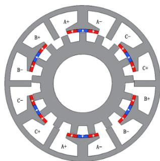
**Figure 7.** Topology of flux reversal motor with three-phase supply [64]. A, B and C represent the three-phase windings of the motor installed in an X configuration.
