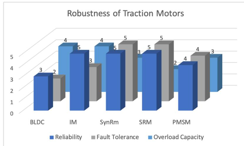
Figure 15. Reliability, stress tolerance and overload capacity scoring for the five selected powertrains.
