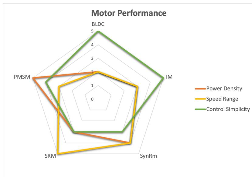
Figure 16. Performance analysis of studied motors based on speed, power and control.
