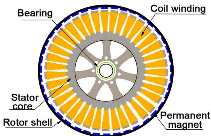
Figure 4. Brushless motor inner design by [37].
