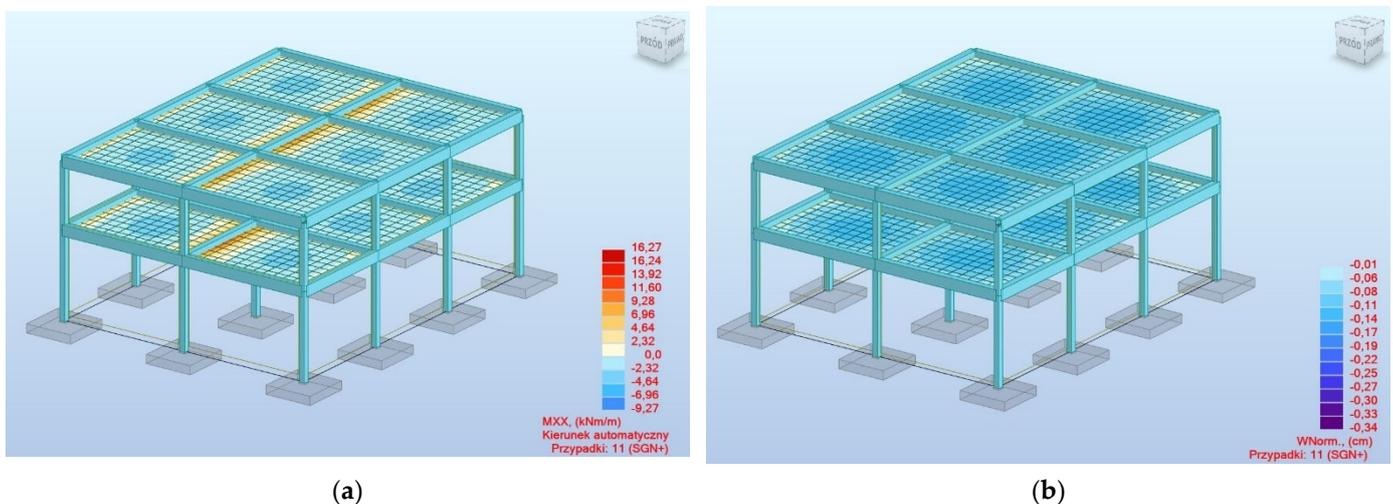
**Figure 6.** Examples of load combination effects: (a) map of flexural moments in the XX direction for floor slabs in ULS; (b) map of deflections of floor slabs in ULS.
