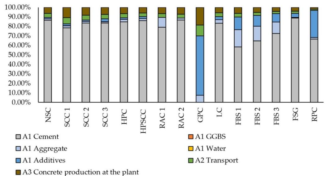
**Figure 8.** Percentage contribution of concrete mix components as well as A2 and A3 phases in the carbon footprint value.
