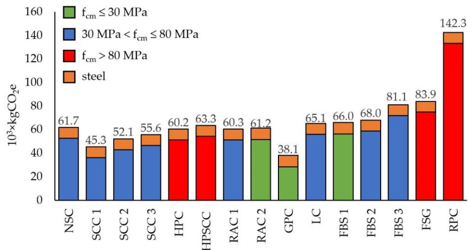
**Figure 11.** Carbon footprint value over the entire life cycle for concrete and reinforcing steel in the analyzed structure.
