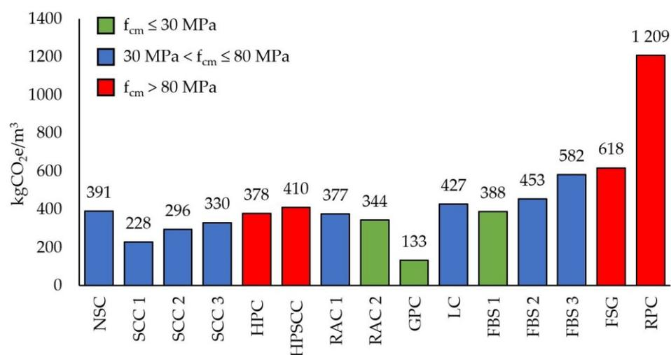
Figure 7. Carbon footprint for phase A1–A3 per 1 m<sup>3</sup> of concrete mix.
