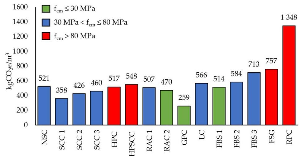
Figure 9. Carbon footprint over the life cycle of concrete per 1 m<sup>3</sup> of concrete mix.
