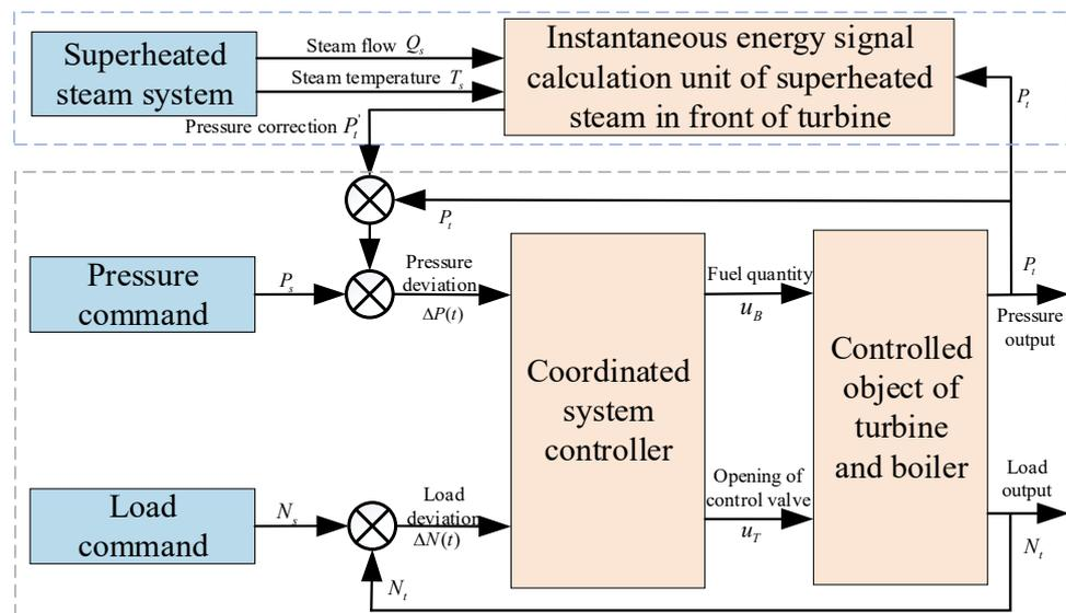
**Figure 7.** Coordination and optimization based on correction of superheated steam energy storage in front of turbine.
