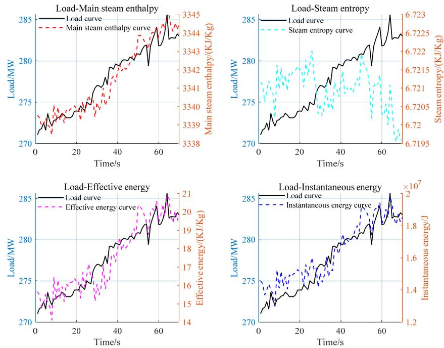
Figure 4. Changes in load and steam energy parameters during load application.
