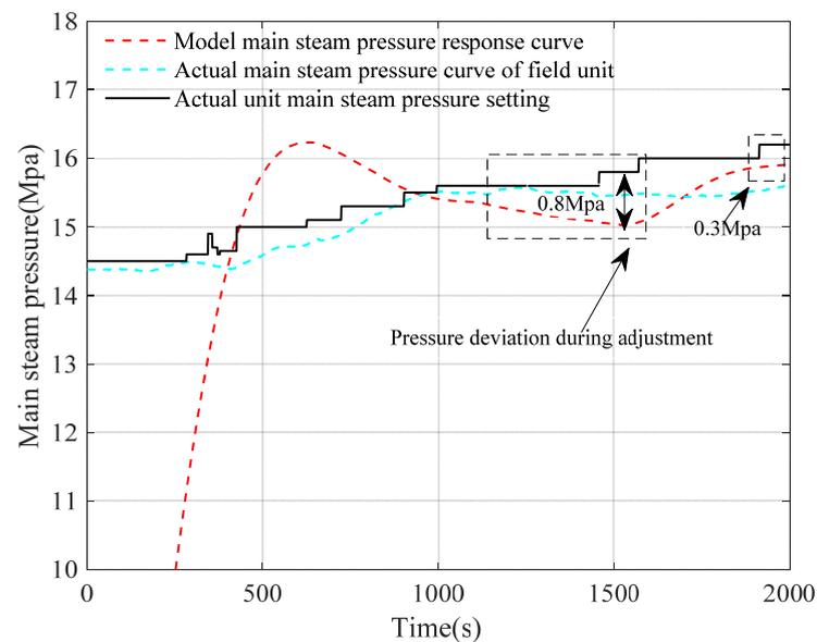
**Figure 11.** Pressure response curve after model optimization and compensation.
