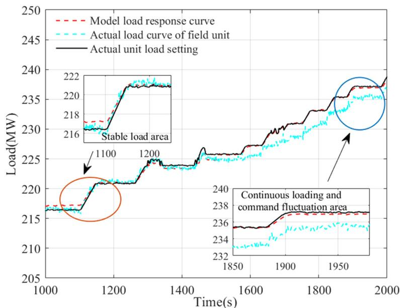
Figure 10. Load response curve after model optimization and compensation.
