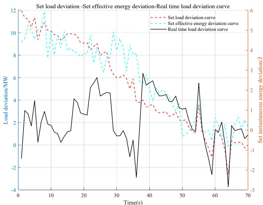
**Figure 6.** Comparison of real-time load deviation between load setting deviation and the available steam energy deviation.
