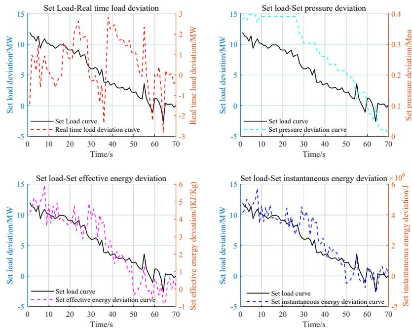
Figure 5. Pressure energy deviation response caused by load tracking during load application.
