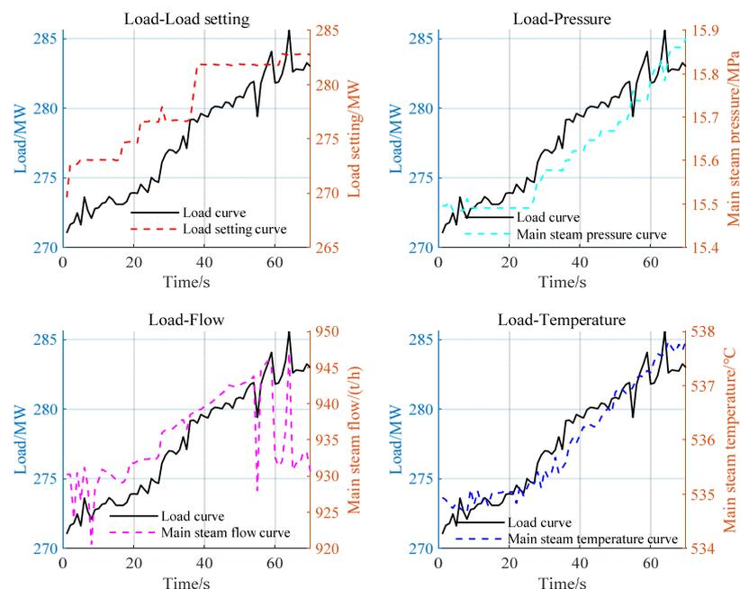
**Figure 3.** Variation between load and main steam parameters during loading.
