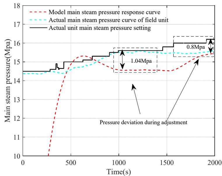
Figure 9. Main steam pressure response curve under traditional modeling mode.
