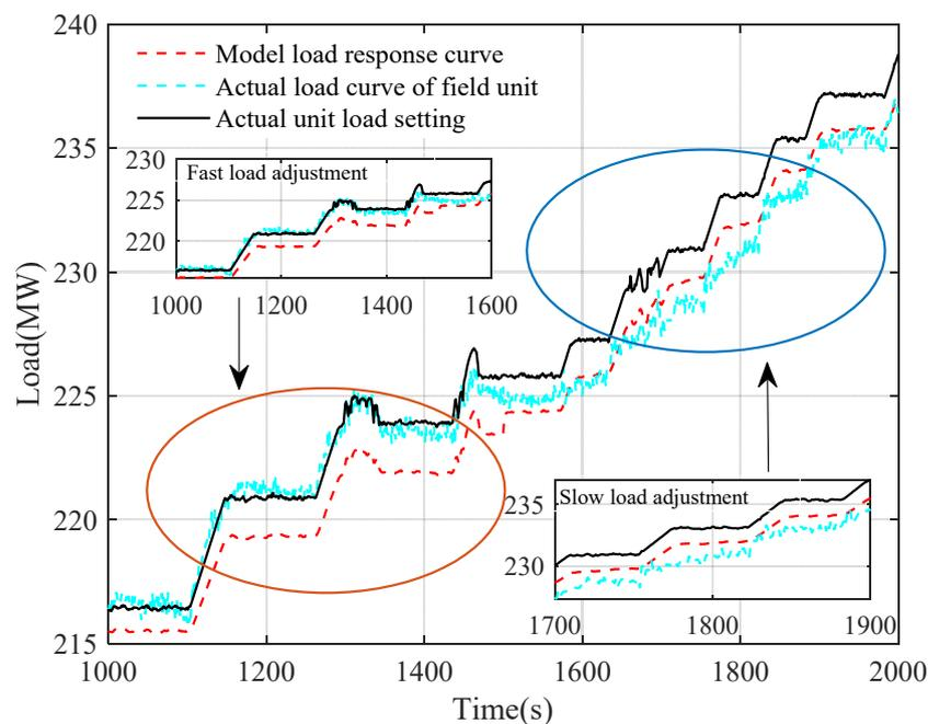
Figure 8. Load response curve under traditional modeling mode.
