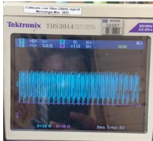
Figure 8. Communication signal between the WEG station and the BYD bus.
