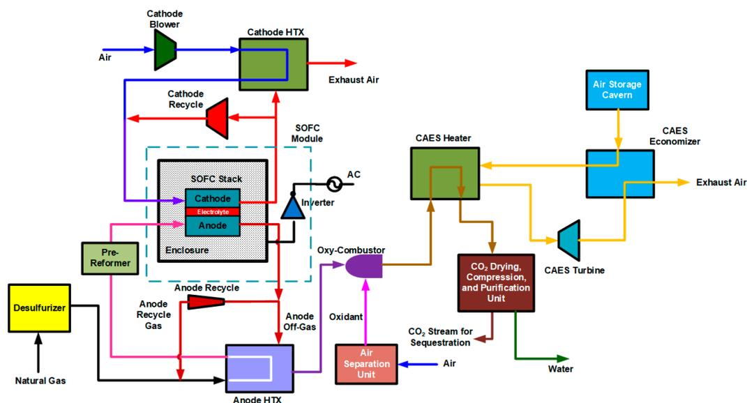
Figure 2. System discharging block flow diagram.
