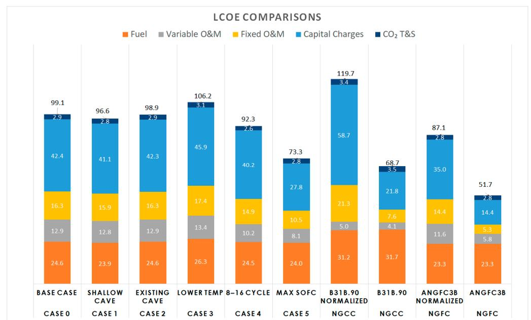
Figure 4. Comparison of LCOE for each case evaluated.
