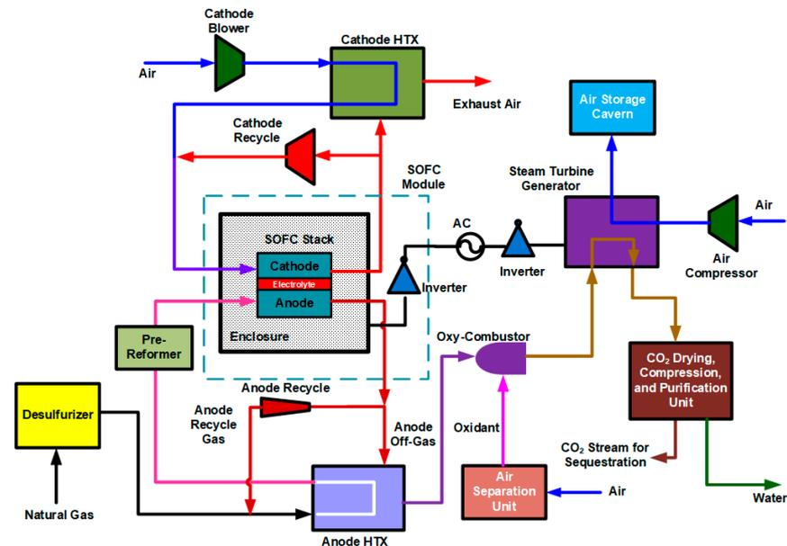
Figure 1. System charging block flow diagram.
