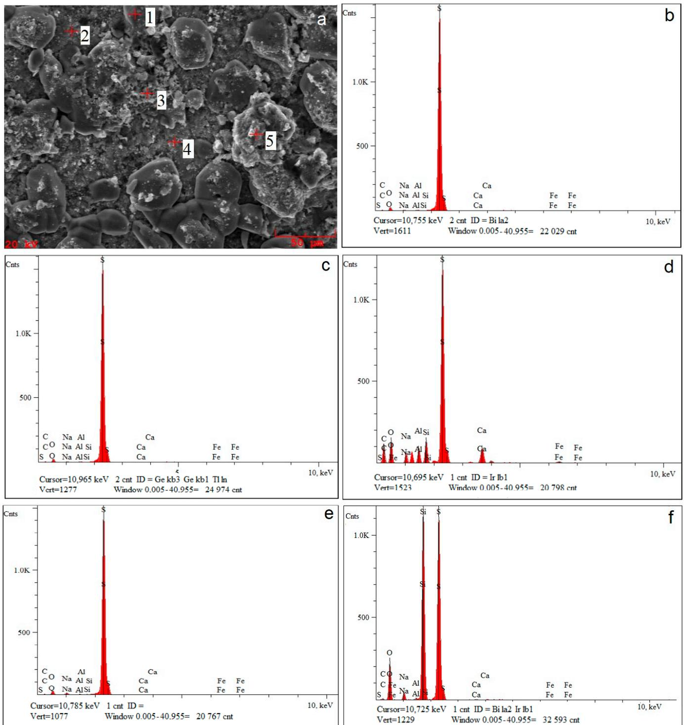
Figure 7. Five-point analysis of a sample of spent activated carbon performed by EDS.
