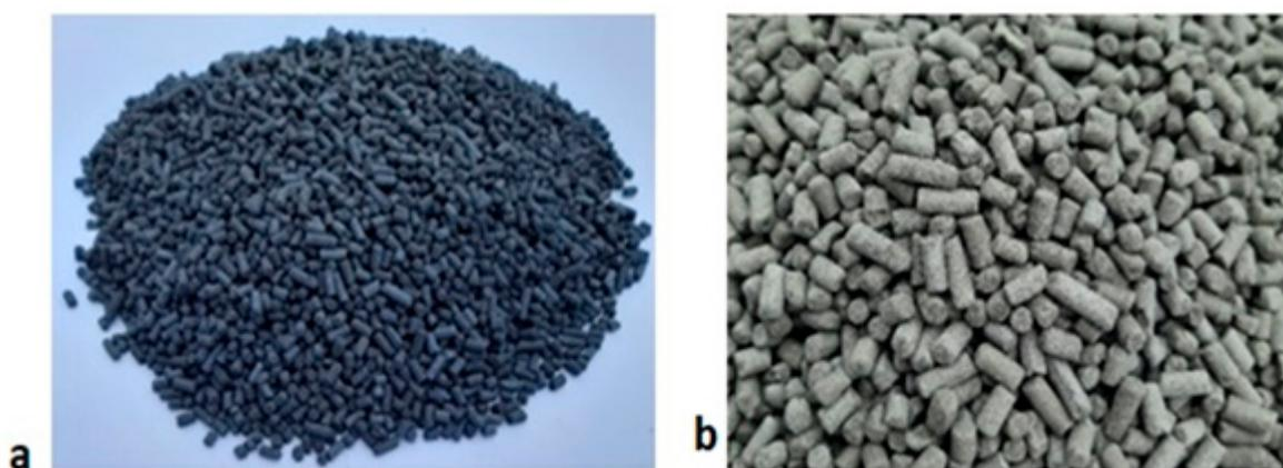
**Figure 2.** Shaped activated carbon: (a) fresh, (b) spent; transferred for laboratory testing.
