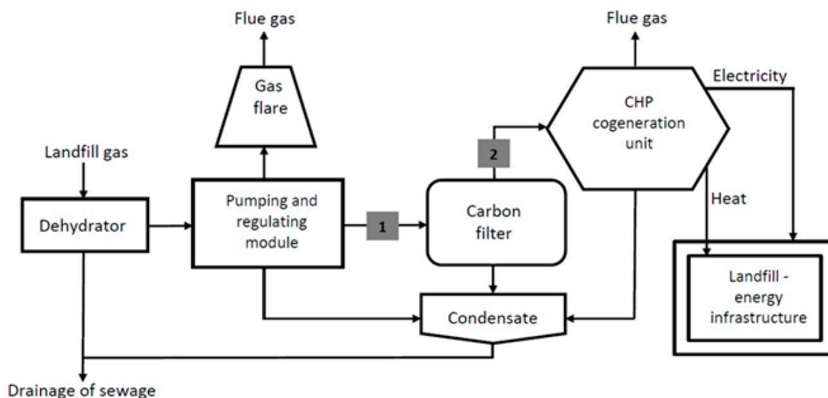
**Figure 1.** Diagram of a landfill gas energy utilisation facility. Own study.
