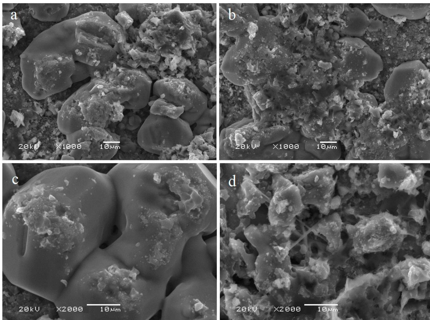
**Figure 6.** Surface images of the activated carbon sample at 1000 (a,b) and 2000 (c,d) magnification.
