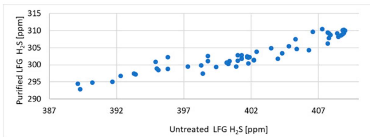
**Figure 3.** H<sub>2</sub>S parameters before activated carbon replacement in the LFG treatment plant.
