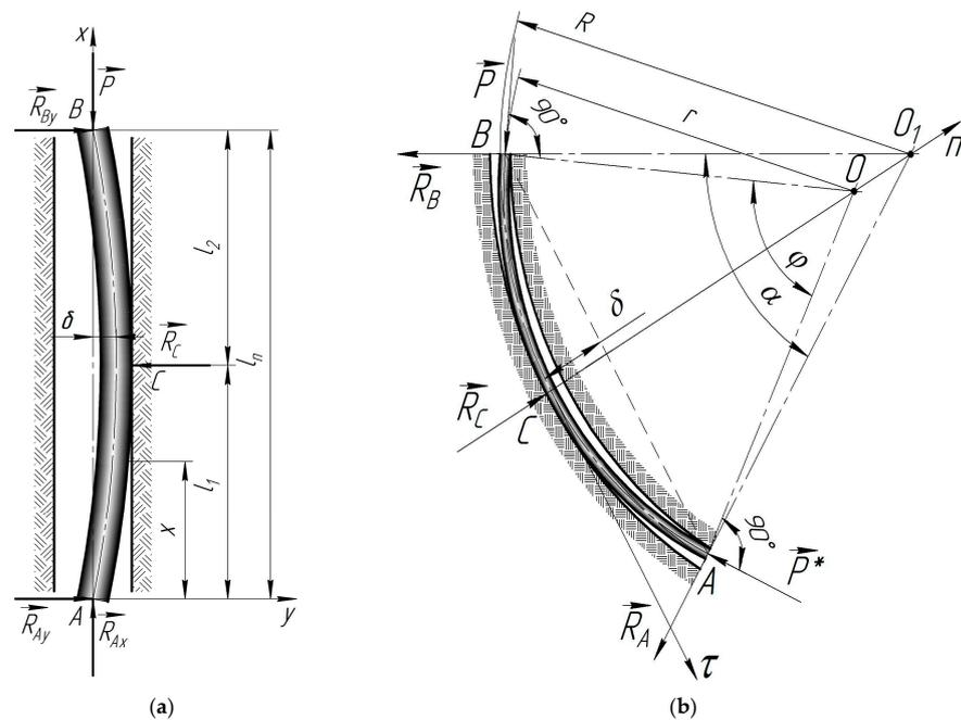
**Figure 1.** Calculation diagram of half-wave loading of a drill string in a conditionally vertical (a) and curved (b) wellbore.
