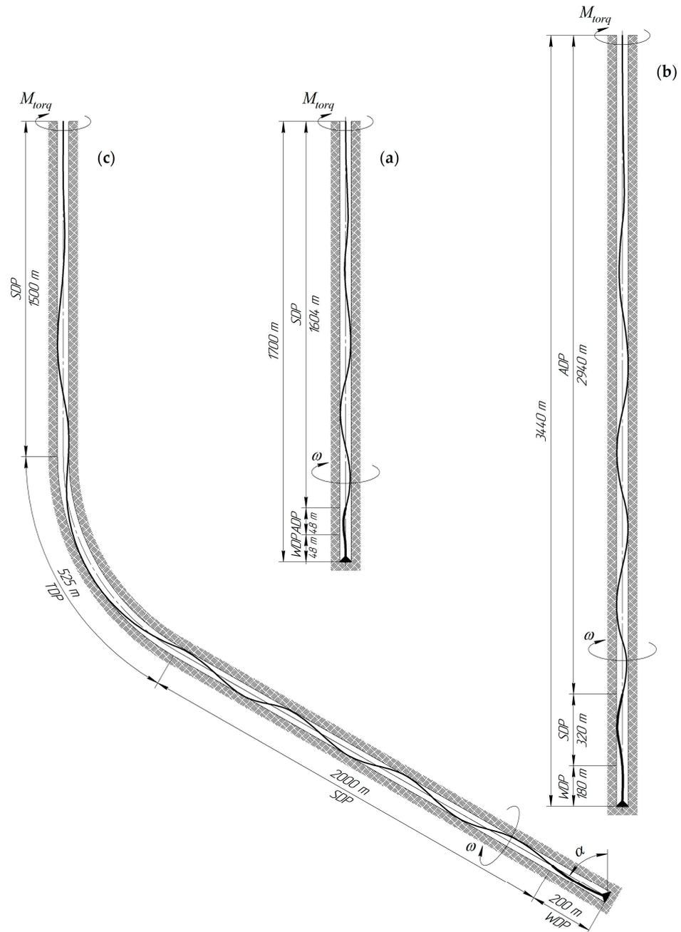
**Figure 3.** Schemes of well profiles and contact of drill strings with the borehole walls for various wells when the design depth is reached: (a) YaK-40; (b) No. 209; (c) Hamad–V.
