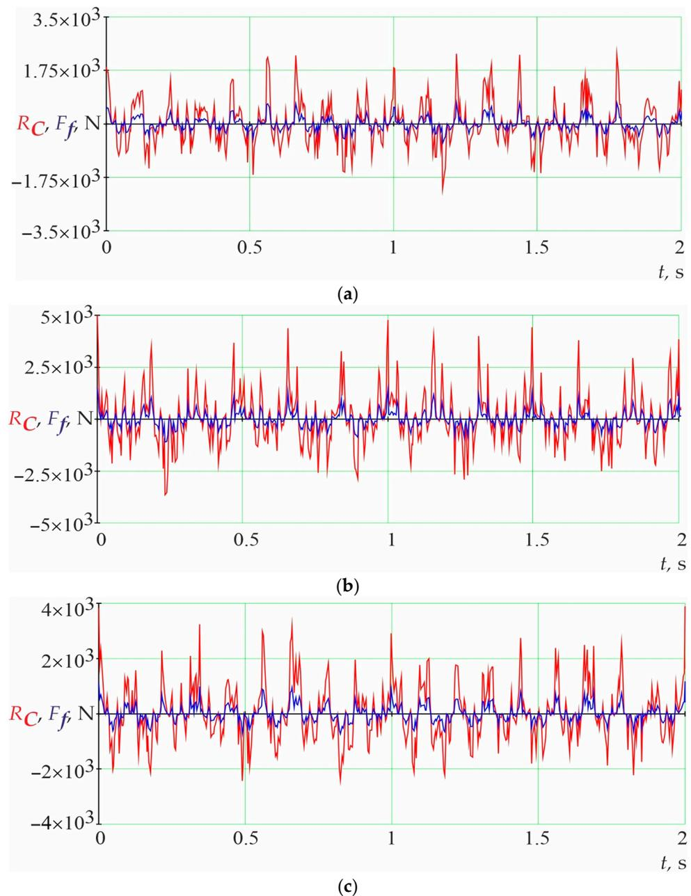
**Figure 5.** Theoretical dependences of the pressure and friction forces of the drill string sections on the borehole walls as a function of time when the design depth is reached: (a) Yak-40,  $L = 1552$  m; (b) No. 209,  $L = 2550$  m; (c) Hamad-V,  $L = 2025$  m.
