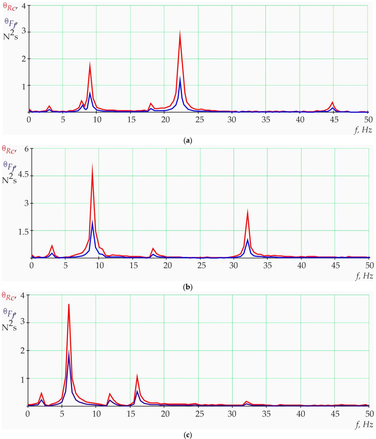
**Figure 6.** Spectral densities of the pressing forces and friction of the drill string sections to the borehole walls when the design depth is reached: (a) Yak-40,  $L = 1552$  m; (b) No. 209,  $L = 2550$  m; (c) Hamad-V,  $L = 2025$  m.
