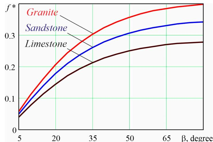
**Figure 2.** The dependence of the effective coefficient of friction refers to the drill string angle of the helix when interacting with various rocks in the well [79].
