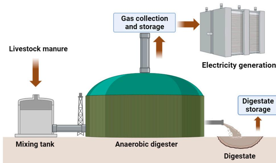
**Figure 3.** Graphical representation of a conventional AD reactor facility for treating livestock manures.
