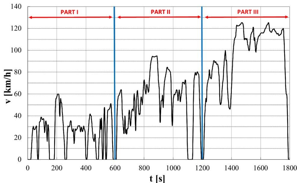
Figure 3. WMTC test [32].
