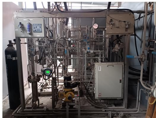
**Figure 5.** Alkaline water electrolyzer of the system in the laboratory.
