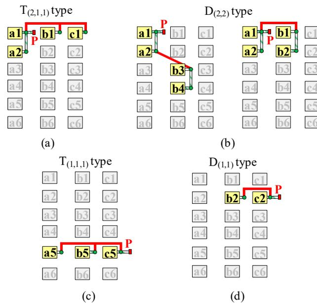
**Figure 12.** Structure of LVDC ports in MPETs shown in Figure 13. (a) Port 1 of  $T_{(2,1,1)}$  type. (b) Port 1 of  $D_{(2,2)}$  type. (c) Port 1 of  $T_{(1,1,1)}$  type. (d) Port 1 of  $D_{(1,1)}$  type.
