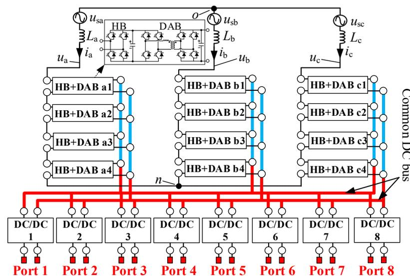
**Figure 2.** Common DC bus structure multiport power electronic transformer (CDBS-MPET).
