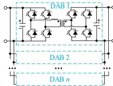
**Figure 3.** Structure of DC/DC 1 to 8 in CDBS-MPET.
