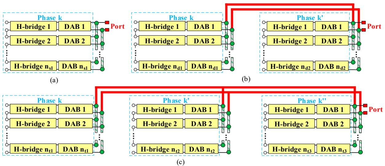
**Figure 5.** Basic structures of LVDC ports. (a) Single-phase connection port (S-Port). (b) Double cross-phase connection port (D-Port). (c) Triple cross-phase connection port (T-Port).
