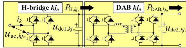
Figure 8. Structure of H-bridge and DAB.
