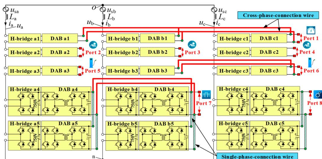
Figure 1. Independent DC bus structure multiport power electronic transformer (IDBS-MPET).
