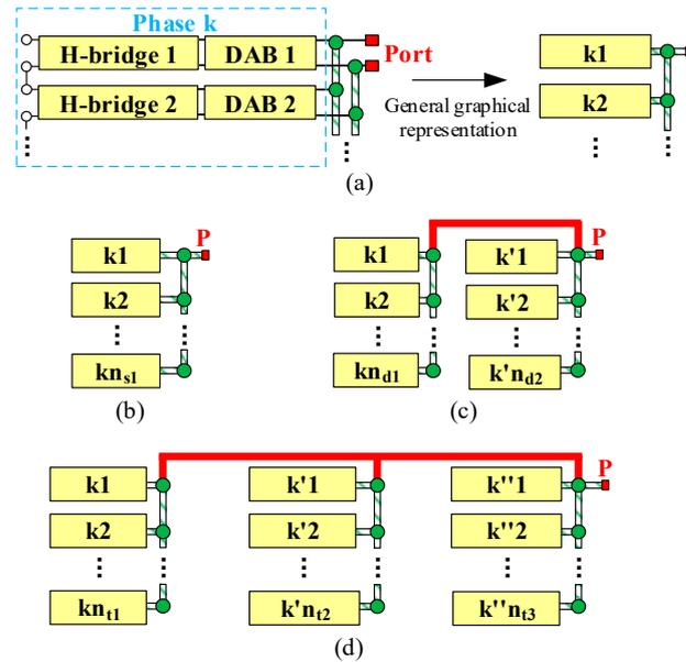
Figure 6. Graphical representation of LVDC ports. (a) General graphical representation of cascaded H-bridge and DAB. (b) S-Port. (c) D-Port. (d) T-Port.
