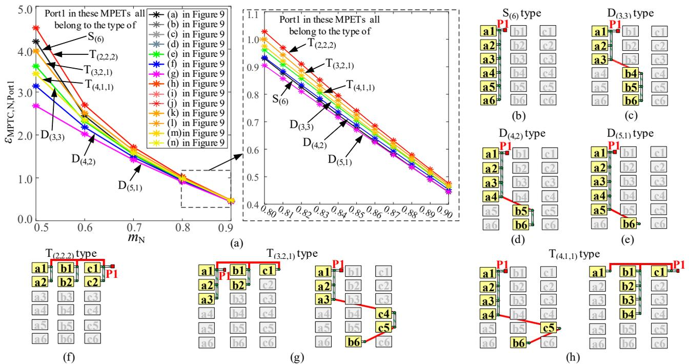
**Figure 10.** MPTC and the structures of Port 1 in MPETs shown in Figure 9. (a) MPTC of Port 1. (b) Port 1 of  $S_{(6)}$  type. (c) Port 1 of  $D_{(3,3)}$  type. (d) Port 1 of  $D_{(4,2)}$  type. (e) Port 1 of  $D_{(5,1)}$  type. (f) Port 1 of  $T_{(2,2,2)}$  type. (g) Port 1 of  $T_{(3,2,1)}$  type. (h) Port 1 of  $T_{(4,1,1)}$  type.
