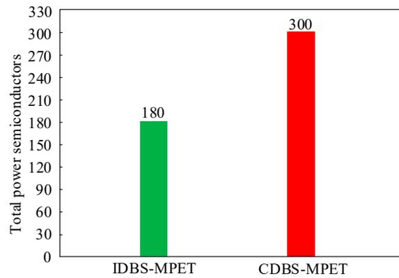
**Figure 4.** Total number of power semiconductors in IDBS-MPET and CDBS-MPET.
