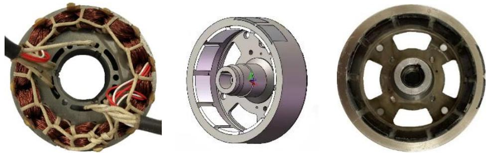
Figure A2. Physical diagram of the generator rotor (left) and structural design diagram of the stator (middle) and physical diagram (right).
