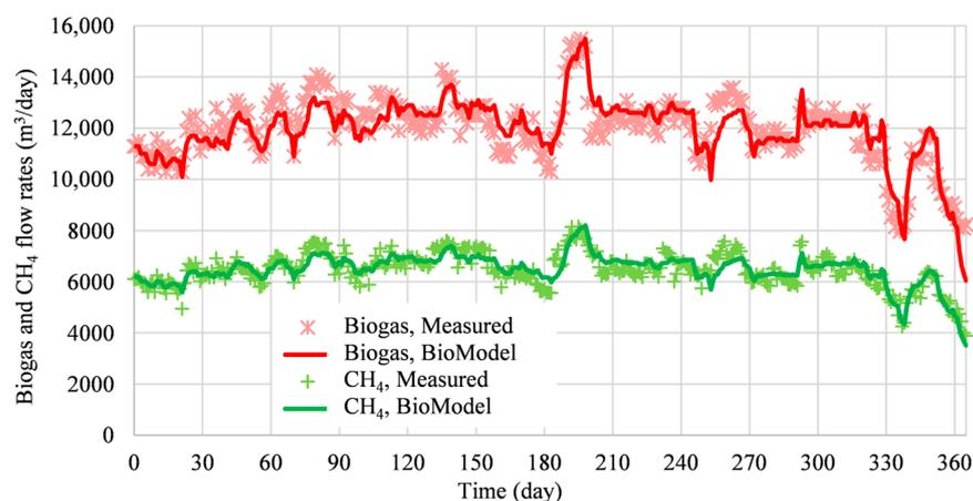
**Figure 3.** Biogas and methane flow rates.
