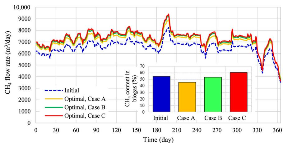
**Figure 8.** Initial and optimized  $CH_4$  flow rates.
