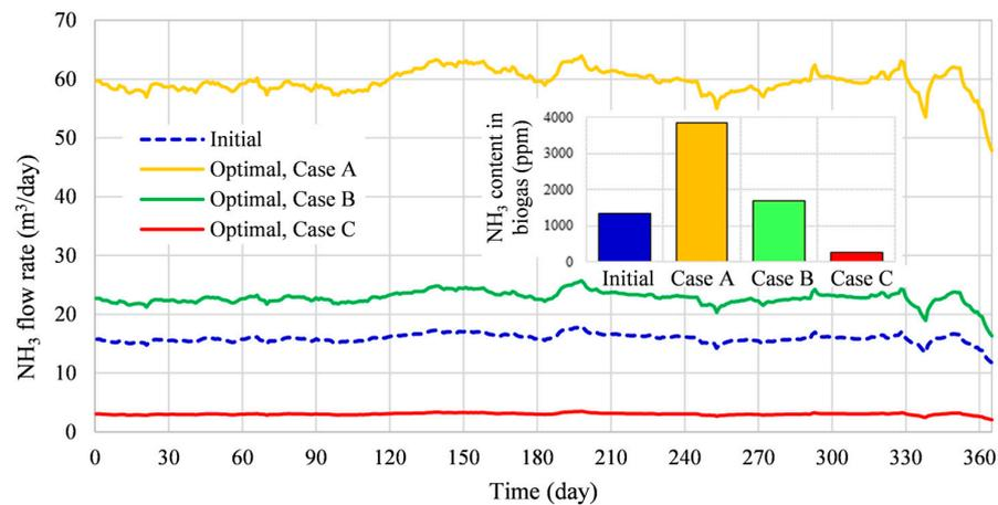
**Figure 11.** Initial and optimized  $\text{NH}_3$  flow rates.
