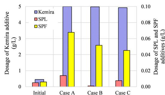
**Figure 6.** Initial and optimized dosages of Kemira BDP-840, SPL, and SPF additives.
