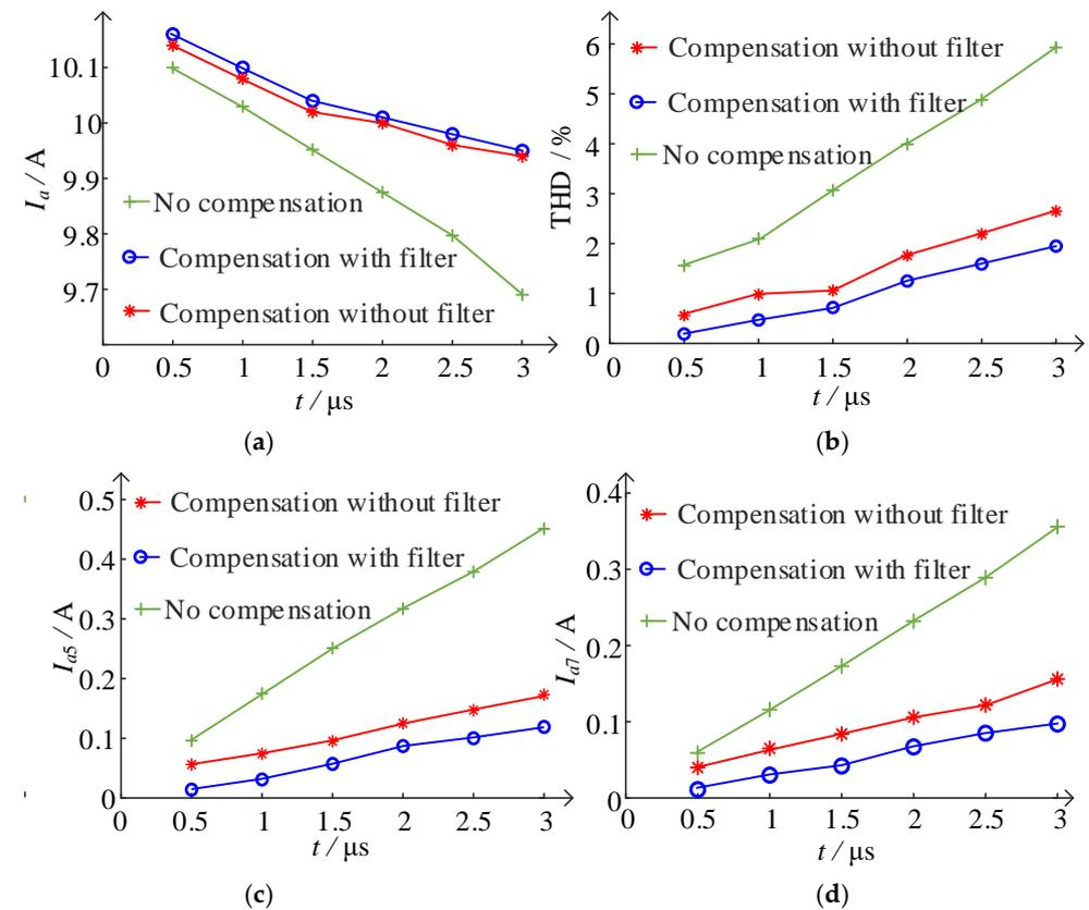
**Figure 20.** The comparison results of no compensation, compensation without discrete filter, and the proposed compensation under different overlap time: (a) fundamental amplitude; (b) THD; (c) amplitude of fifth harmonic; (d) amplitude of seventh harmonic.
