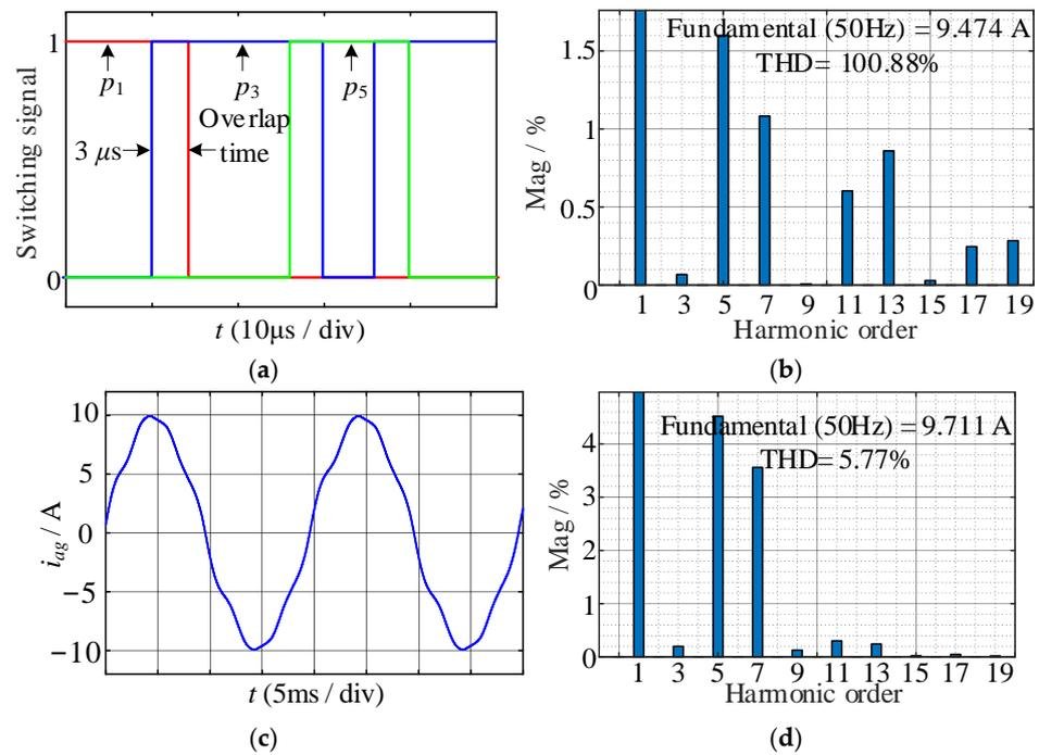
**Figure 13.** Simulation results with overlap time of 3  $\mu$ s: (a) switching signals; (b) FFT results of  $i_a$ ; (c)  $i_{ag}$ ; (d) FFT results of  $i_{ag}$ .
