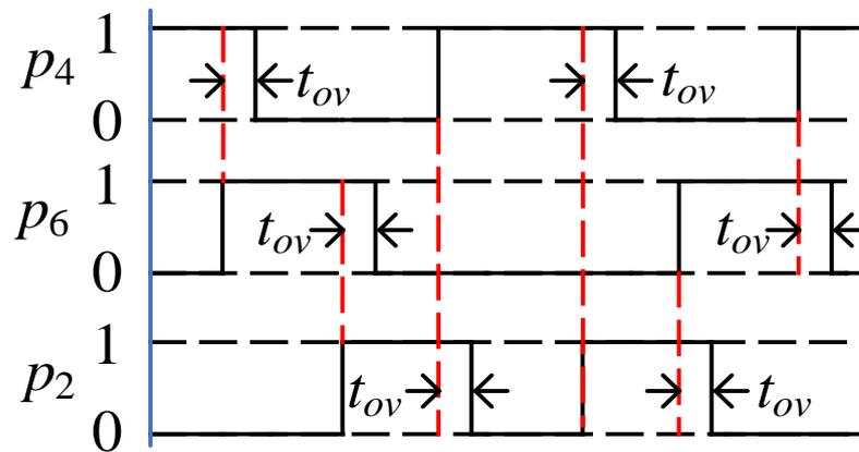
**Figure 4.** Switching signals diagrams with overlap time.
