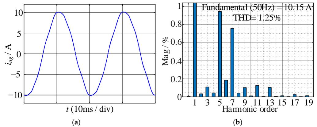
**Figure 15.** Simulation results after compensation under  $t_{ov} = 3 \mu\text{s}$ : (a) waveform of  $i_{ag}$ ; (b) FFT results of  $i_{ag}$ .
