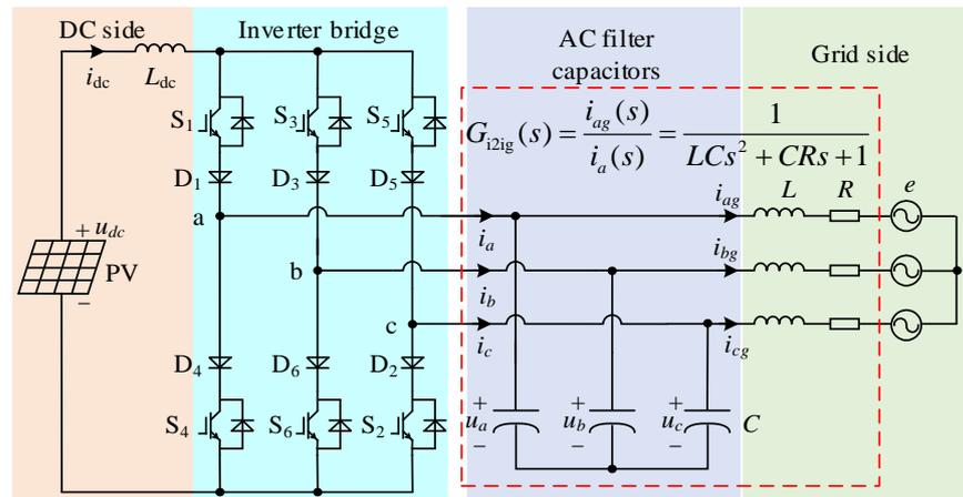
Figure 1. Topology of the current source PV grid-connected inverter.
