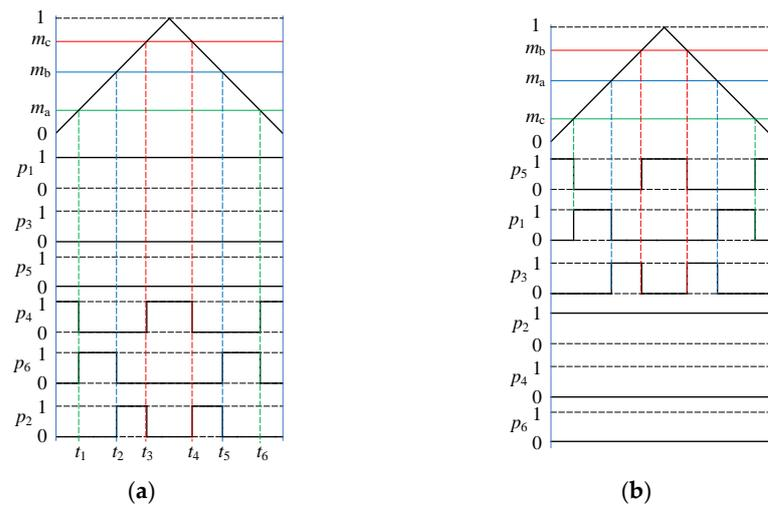
**Figure 3.** Switching signals diagrams in a carrier period under seven-segment SVM: (a) sector I; (b) sector II.
