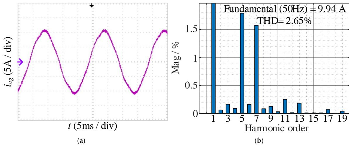
**Figure 19.** Experimental results with compensation and no discrete filter under  $t_{ov} = 3 \mu s$ : (a) waveform of  $i_{ag}$ ; (b) FFT results of  $i_{ag}$ . Purple arrow—the zero tick mark.
