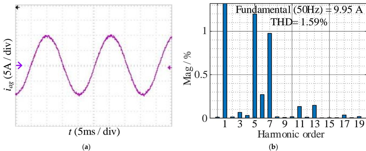
**Figure 18.** Experimental results with compensation under  $t_{ov} = 3 \mu\text{s}$ : (a) waveform of  $i_{ag}$ ; (b) FFT result of  $i_{ag}$ . Purple arrow—the zero tick mark.
