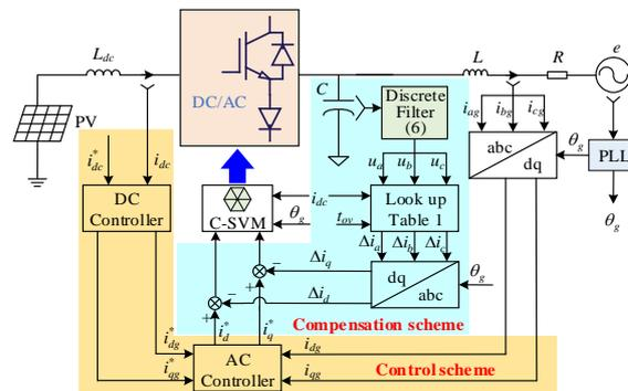
Figure 10. Control structure with compensation of the overlap time.
