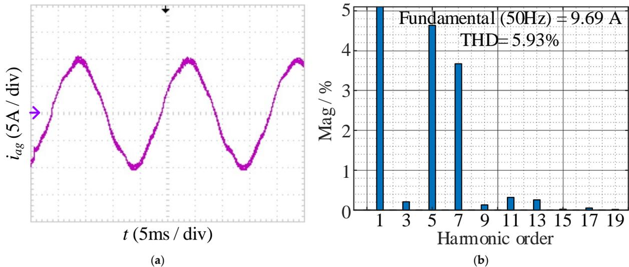
**Figure 17.** Experimental results without compensation under  $t_{ov} = 3 \mu\text{s}$ : (a) waveform of  $i_{ag}$ ; (b) FFT result of  $i_{ag}$ . Purple arrow—the zero tick mark.
