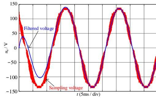
Figure 11. The waveforms of  $u_a$  before and after the discrete filter.
