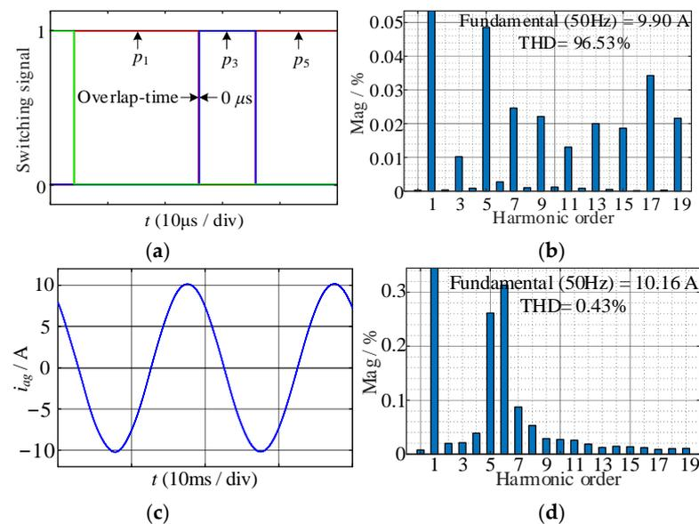
Figure 12. Simulation results without overlap time: (a) switching signals; (b) FFT results of  $i_a$ ; (c)  $i_{ag}$ , (d) FFT results of  $i_{ag}$ .
