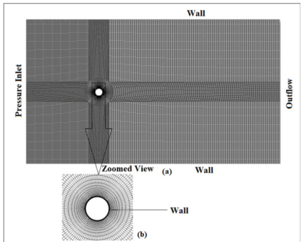
**Figure 6.** (a) Computational mesh; (b) zoomed view of mesh around the cylinder.
