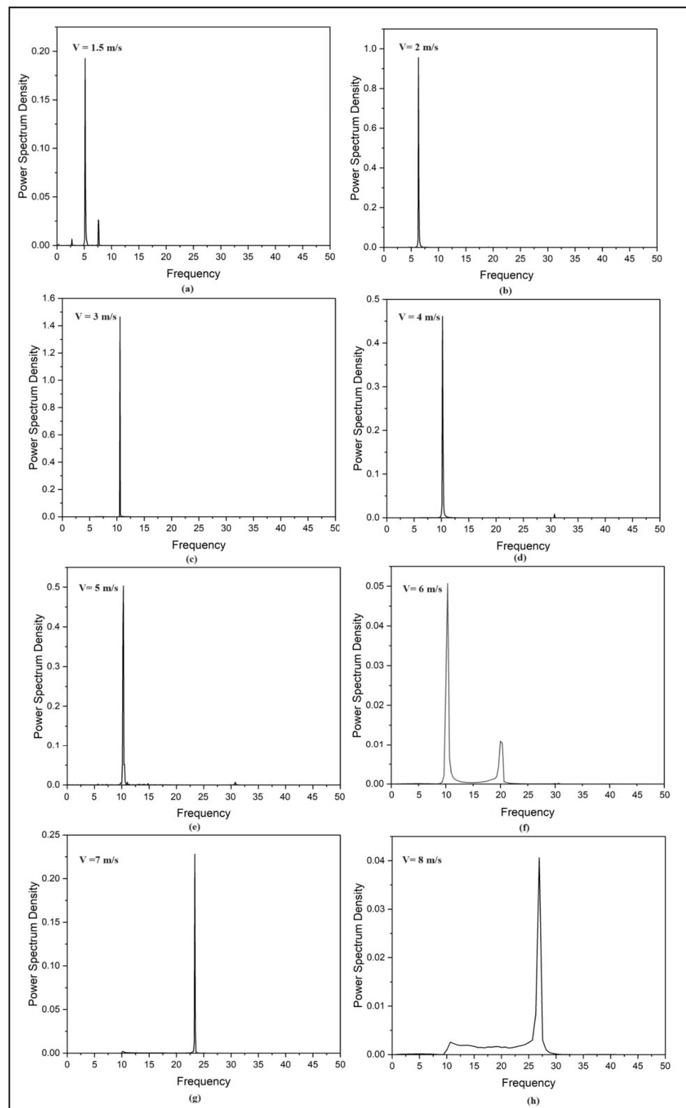
**Figure 13.** Power spectrum density of coefficient of lift for various wind speeds  $V$  (linear system) versus frequency (Hz), (a) 1.5 m/s, (b) 2 m/s, (c) 3 m/s, (d) 4 m/s, (e) 5 m/s, (f) 6 m/s, (g) 7 m/s, & (h) 8 m/s.
