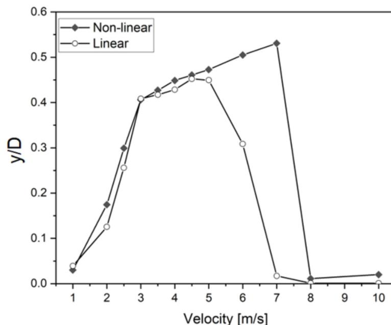
**Figure 7.** Variations in the cylinder response amplitude with wind velocity for linear and nonlinear springs.
