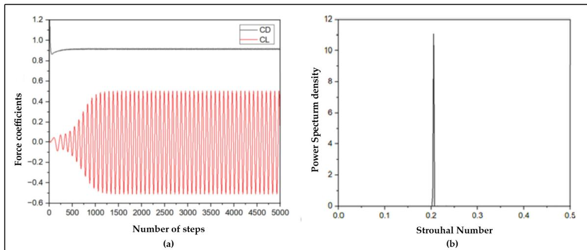
**Figure 3.** (a) Force coefficient (CD—drag coefficient; CL—lift coefficient) time series (expressed in the time sampling steps) and (b) corresponding power spectrum density against the Strouhal number at  $Re = 10,000$ .
