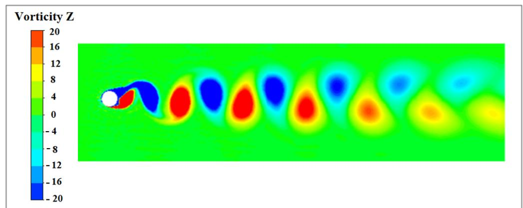
Figure 2. Instantaneous wake structure (Z-vorticity) for flow past fixed cylinder at  $Re = 10,000$ .
