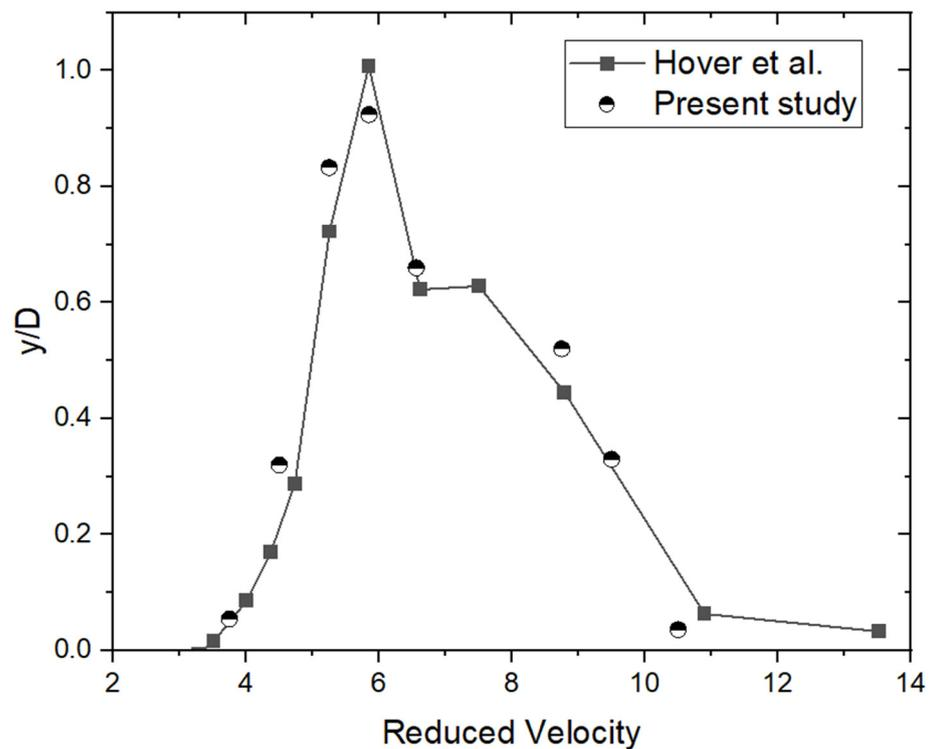
**Figure 4.** Comparison of response amplitude with experimental data (Hover et al. [26]) at  $Re = 10,000$ .
