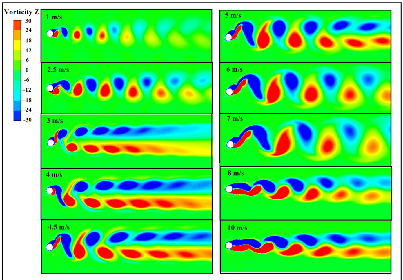
**Figure 9.** Vorticity contours at selected wind velocities for a nonlinear spring force.
