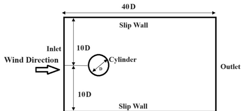
Figure 1. Two-dimensional geometry with boundary conditions.
