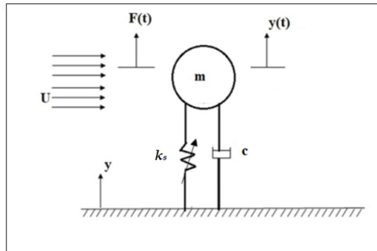
**Figure 5.** Sketch of elastically mounted cylinder in fluid flow. The nonlinear spring is practically realized as the cantilever beam.
