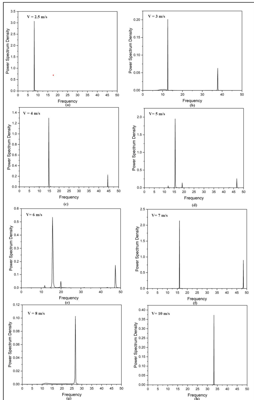
**Figure 14.** Power spectrum density of coefficient of lift for various wind speeds  $V$  (cubic nonlinear system) versus frequency (Hz), (a) 2.5 m/s, (b) 3 m/s, (c) 4 m/s, (d) 5 m/s, (e) 6 m/s, (f) 7 m/s, (g) 8 m/s, & (h) 10 m/s.
