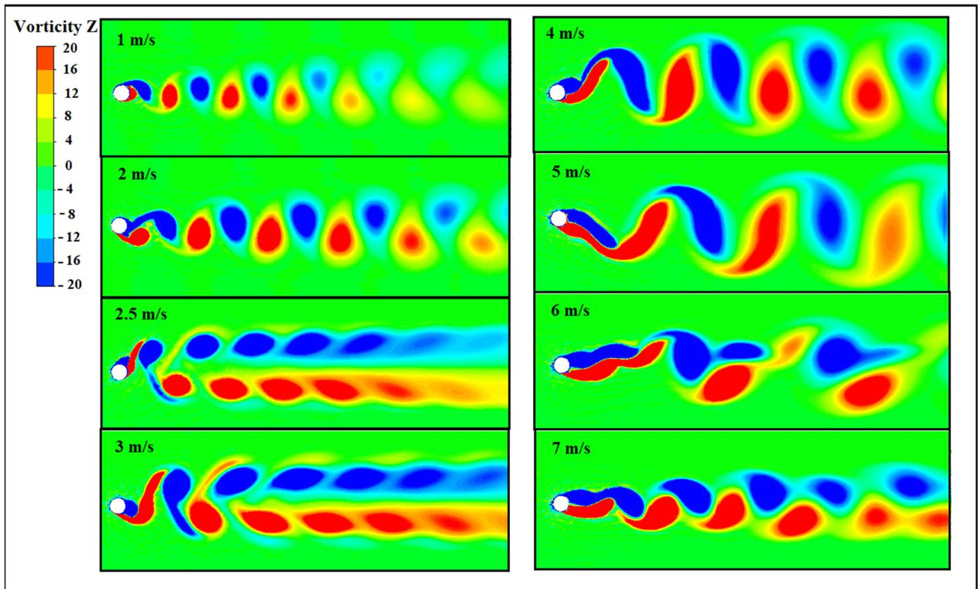
**Figure 8.** Vorticity contours at selected wind velocities for a linear spring force.
