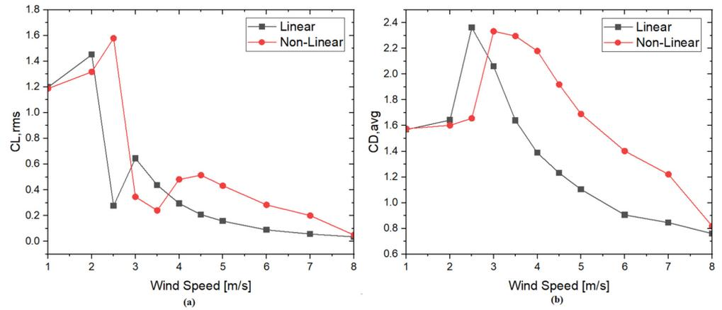
**Figure 10.** Force coefficients on single oscillating cylinder: (a) root-mean-square values of RMS lift coefficient; (b) average drag coefficient.
