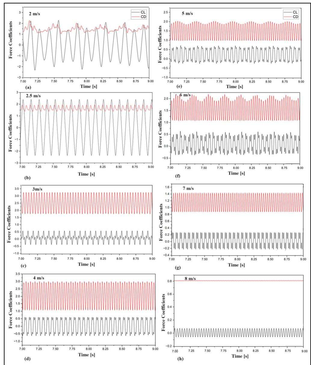
**Figure 12.** Time histories of lift coefficient with various wind speeds (cubic nonlinear system), (a) 2 m/s, (b) 2.5 m/s, (c) 3 m/s, (d) 4 m/s, (e) 5 m/s, (f) 6 m/s, (g) 7 m/s, & (h) 8 m/s.
