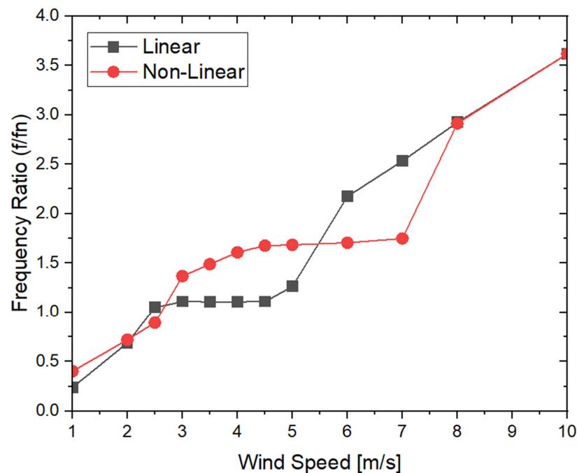
Figure 15. Frequency ratio of oscillating cylinder for linear system and nonlinear system.
