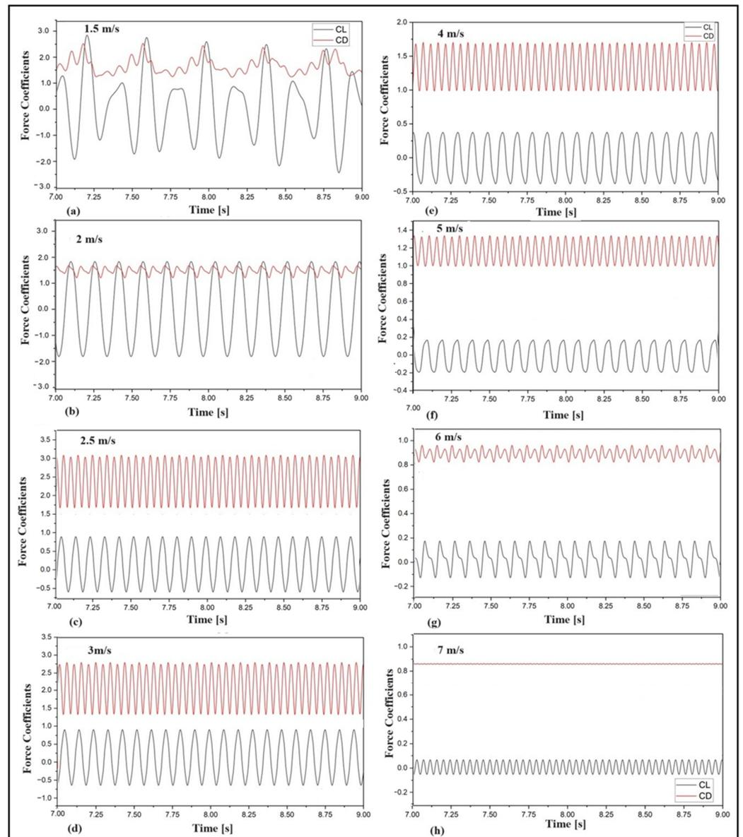
**Figure 11.** Time histories of lift coefficient with various wind speeds (linear system of the mechanical structure), (a) 1.5 m/s, (b) 2 m/s, (c) 2.5 m/s, (d) 3 m/s, (e) 4 m/s, (f) 5 m/s, (g) 6 m/s, & (h) 7 m/s.
