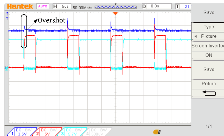
Figure 21. Output voltage PWM signals for both MOSFETs used PID controller.
