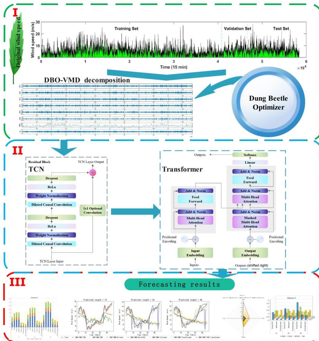
Figure 1. Flowchart of the developed model.
