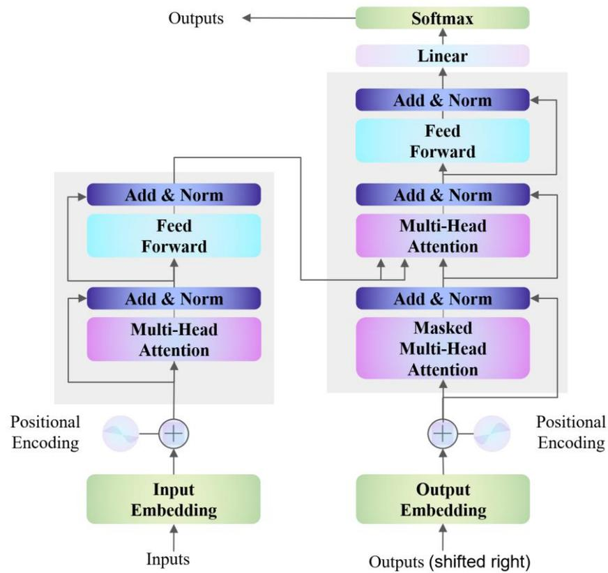
Figure 3. The transformer architecture.
