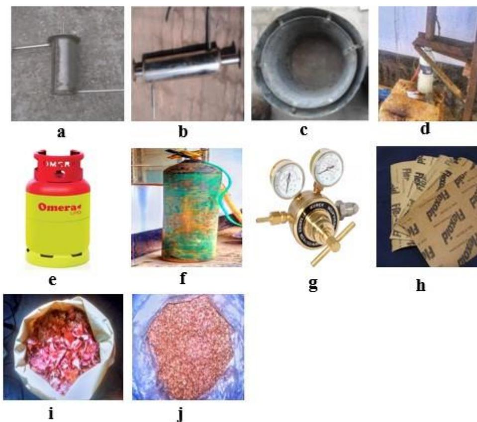
**Figure 1.** Different parts of the fixed-bed pyrolysis setup; (a) Reactor; (b) Condenser; (c) Biomass heater; (d) Liquid collector; (e) LPG cylinder; (f)  $N_2$  gas cylinder; (g) MUREX 57 series gas flow meter; (h) Liquid gasket; (i) Onion shell; (j) Feed materials with average particles size of  $200\text{--}300\text{ }\mu\text{m}$ .
