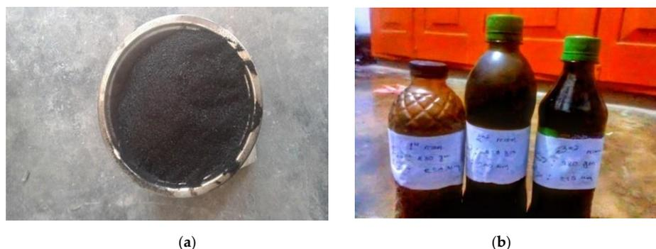
**Figure 3.** (a) Produced char. (b) Produced oil from onion shell pyrolysis.
