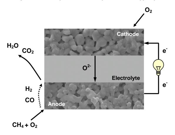
Figure 3. Schematic representation of the single-chamber working principle.
