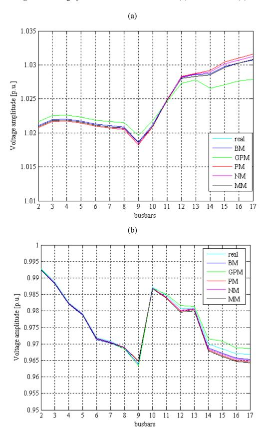
Figure 8. Voltage profile of the network at hour 19 (a) and at hour 20 (b).
