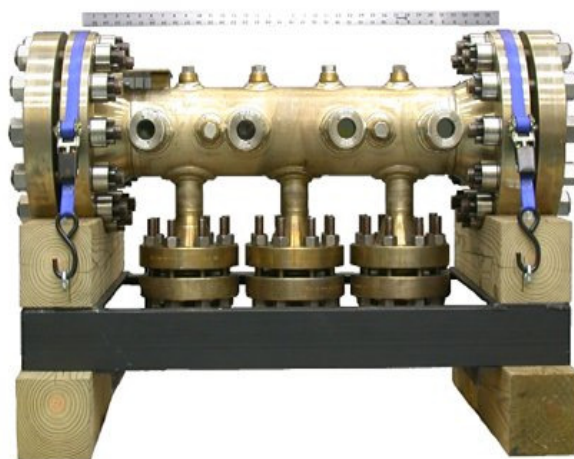
Figure 11. NETL 15-Liter Hydrate Cell; horizontal installation with viewports (4 Cameras) along equator, and numerous instrumentation ports throughout the cell.
