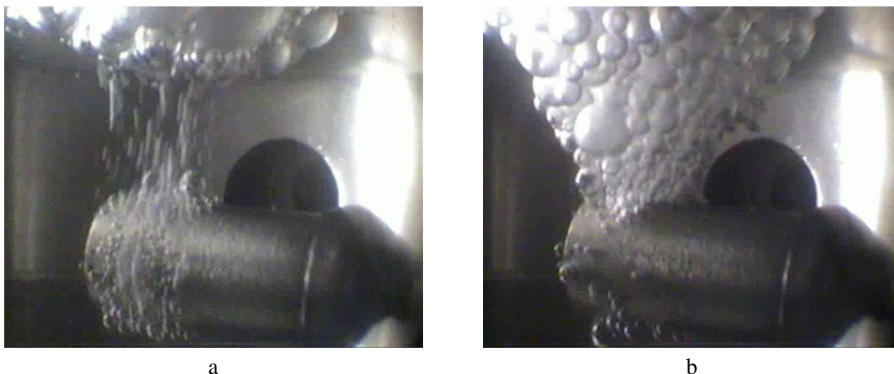
Figure 9. (a) Methane injection through a sintered filter into water; (b) methane injection through a sintered filter into water.
