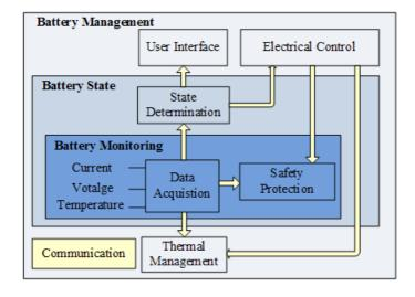
Figure 1. Illustration of a battery management system.
