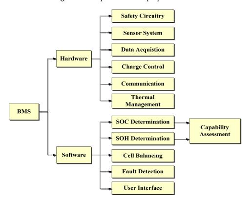
**Figure 3.** Components of the proposed BMS.
