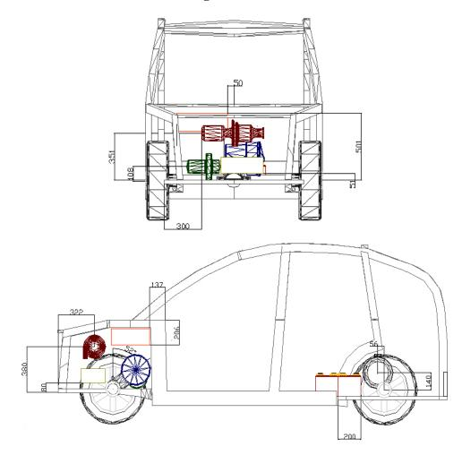
Figure 10. Weight distribution in the LETHE<sup>™</sup> City Car configuration.
