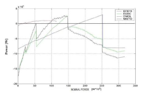
Figure 1. Energy balance as function of installed GT power and track [1].
