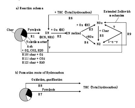
**Figure 3.** Reaction model of  $NO_x$  formation and reduction.
