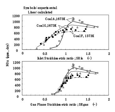
Figure 5. Comparison between measured (symbols) and calculated (line) NO<sub>x</sub> concentrations.
