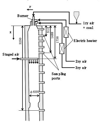
Figure 7. Schematic diagram of the laboratory scale furnace (unit: mm).
