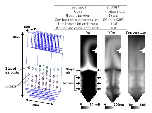
Figure 13. Numerical calculation for oxyfuel combustion.
