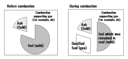
Figure 1. Definition of gas phase stoichiometric ratio (SRgas).
