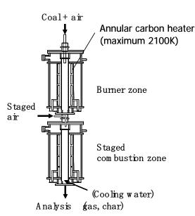
Figure 16. Structure of the drop-tube furnace for staged combustion.
