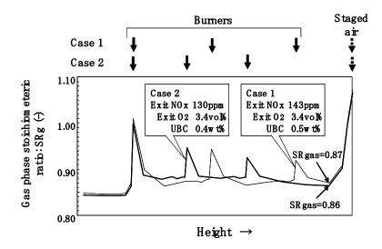
The burner arrangements for CASE 1 and CASE 2 are described in Figure 15. Areas shown by dotted lines represent the main combustion region. Much of the supplied coal burned in this area. Much of the supplied heat was released in the area too. Total heat input of CASE 1 and CASE 2 were
