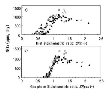
Figure 2. Relationship between gas phase stoichiometric ratio and NO<sub>x</sub> concentration.
