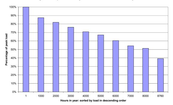
Figure 6. System load profile for Sabah electrical grid.
