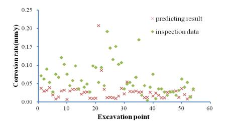
Figure 6. The predicted results and the inspection data of the validation pipeline.
