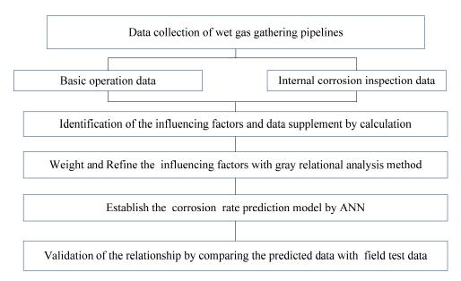
Figure 1. The logic diagram used to establish the method.
