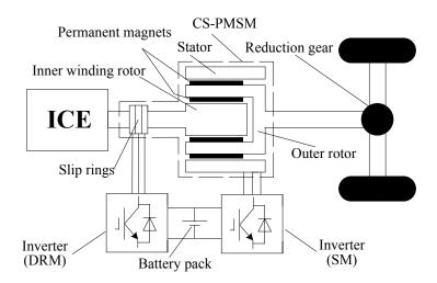
Figure 1. Hybrid electric system based on CS-PMSM.
