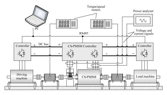
Figure 7. CS-PMSM test bench.
