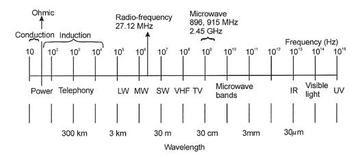
**Figure 1.** Typical electromagnetic spectrum with examples of applications performed at different frequency ranges [32].
