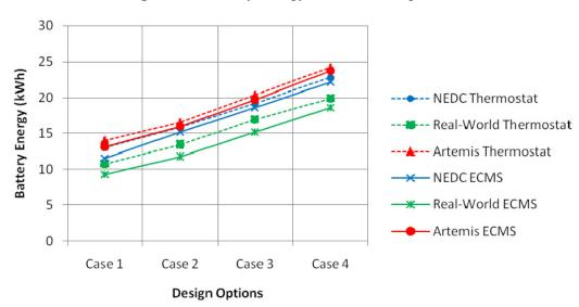
Figure 16. Battery energy for different options.
