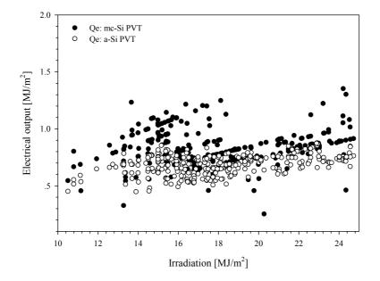
Further measurement of PVT performance is required to elaborate the experimental expression on the relationship between energy output and solar irradiation.
