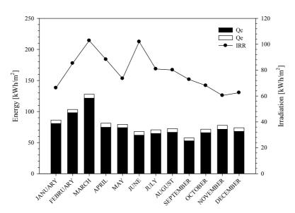
Figure 10. Energy production of a-Si PVT collector.
