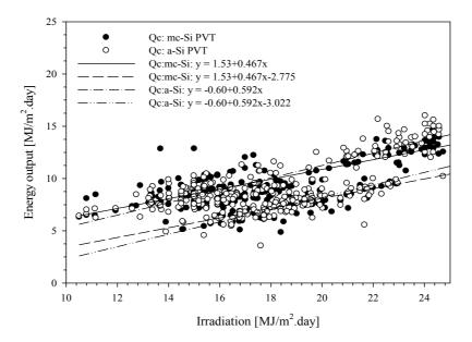
Figure 15 shows the electrical outputs versus solar irradiation, the plots show that the electricity production slightly increases with the solar irradiation. The figure also shows that the electrical production of mc-Si PVT seems scattered than that of a-Si PVT. With these experimental results, the energy output of PVT systems can be roughly estimated based on the solar irradiation except for June because of the rainy season in Thailand.
