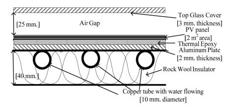
Figure 2. Cross sectional PVT collector.
