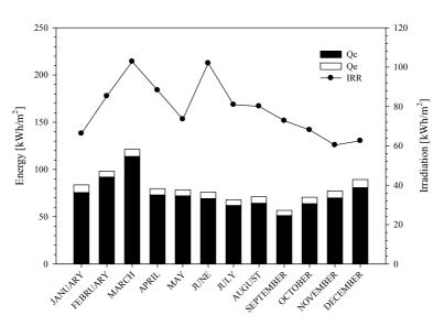
Figure 11. Energy production of mc-Si PVT collector.
