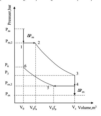
**Figure 2.** PV diagram representing the internal expansion process.
