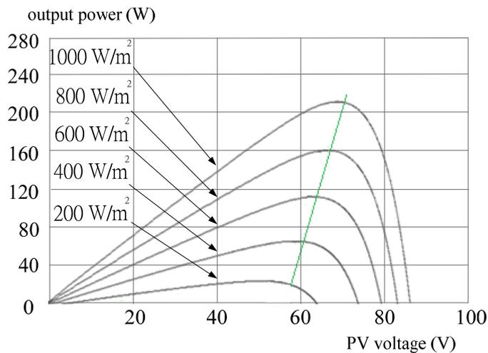
**Figure 12.** The MPPT trajectory by the POM under constant irradiation.
