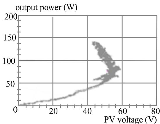
**Figure 17.** Practical measurement of the PV power system with the DLAA.
