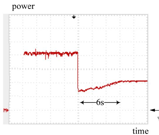
**Figure 25.** Practical measurement: tracking trajectory of the converter with the DLAA while PV power steps down from 200 to 100 W. Note: power: 50 W/div; time: 0.5 s/div.
