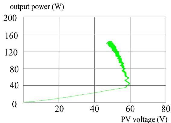
**Figure 15.** MPPT trajectory by the DALL while irradiation and temperature increase.
