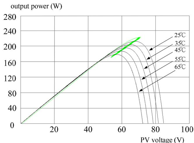
**Figure 13.** MPPT trajectory by the DLAA under constant irradiation.
