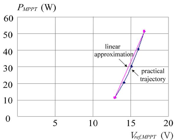
**Figure 5.** The relationship between  $P_{MPPT}$  and  $V_{ref,MPPT}$  while module temperature increases from 25 to 65 °C.
