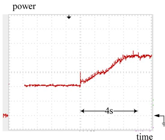
**Figure 23.** Practical measurement: tracking trajectory of the converter with the DLAA while PV power steps up from 100 to 200 W. Note: power: 50 W/div; time: 0.5 s/div.
