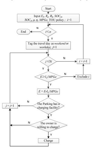
Figure 2. Algorithm used for generation of charging schedules.
