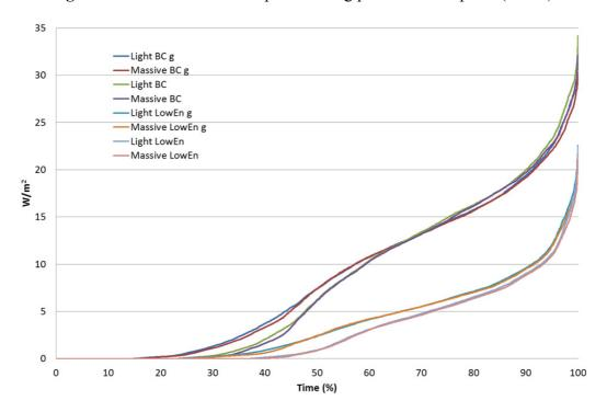
Figure 3. Duration curves of space heating power consumption  $(W/m^2)$ .
