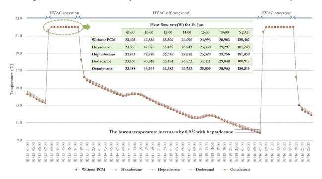
Figure 5. The lowest indoor temperature curve and the heat flow rate for 13 January.
