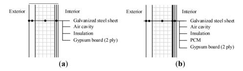
In addition, the material properties were based on the ASHRAE Handbook Fundamentals 2009 (Table 3). The thermal resistances may be affected by the installation of the PCM. To verify that the addition of the PCM does not cause a significant increase in the thermal resistance, the total thermal resistance values of the wall without the PCM and with the PCM are added to Table 3.
