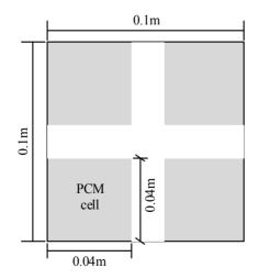
For the input data of the PCM module in EnergyPlus, the PCM cells were assumed to be a continuous layer rather than individual cells. By considering both the mat area and the PCM cells' volume, the thickness of the PCM layer was calculated as follows:
