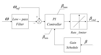
Figure 4. Schematic diagram of pitch angle controller.
