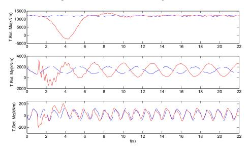
Figure 14. Tower bottom bending moments.
