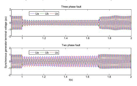
Figure 6. Synchronous generator terminal voltage.
