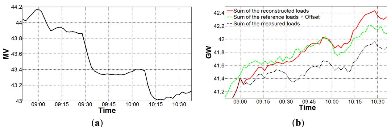
For comparison, 11 April 2013 was selected as the reference date for the reference loads, and an offset of 366 MW was added to the sum of reference loads. As shown in Figure 8b, the maximum peak-load shaving for the first-step voltage reduction took place at 9:54, with a reduction amount of 358 MW. For the second-step voltage reduction, the maximum peak-load shaving took place at 10:20, with a reduction amount of 495 MW.
