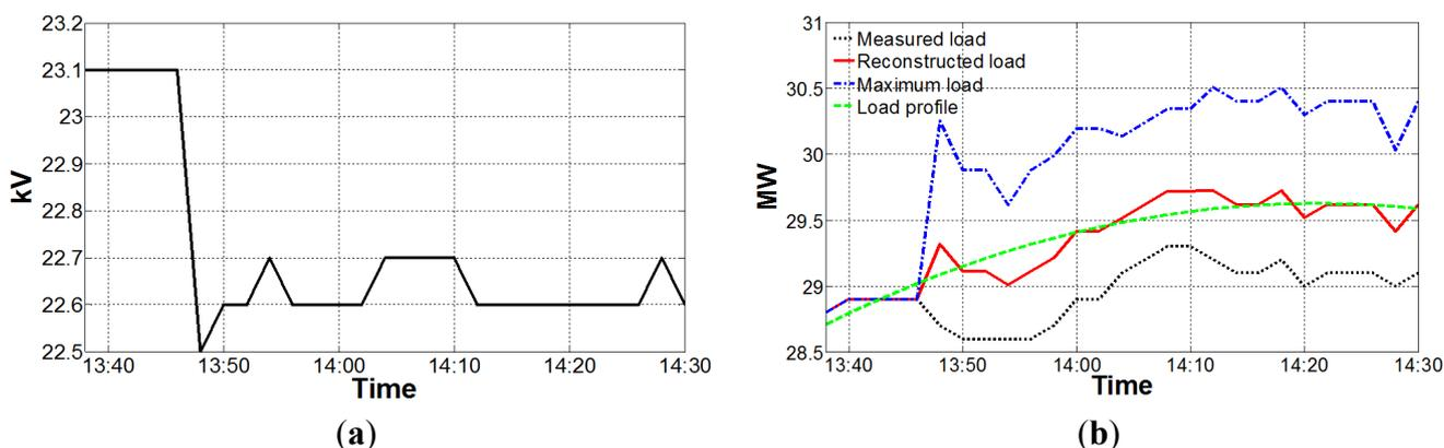
In the case of the 480th transformer bank, the inception time was 13:48 and its actual voltage reduction was about 2.59%, declining from 23.1 kV to 22.5 kV, as shown in Figure 3a. In this case, the objective function of Equation (6) reaches its minimum value when  $p_{C_{480}} = 0.22$ ,  $a_{2_{480}} = -0.00002$ ,  $a_{1_{480}} = 0.01208$ , and  $a_{0_{480}} = 30.2622$ .
