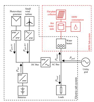
Figure 1. Electrothermal microgrid scheme.
