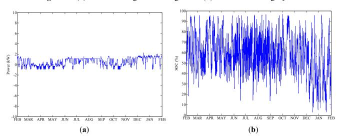
Figure 18. (a) Power exchanged with the grid and (b) useful SOC during a year.
