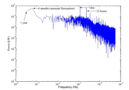
Figure 3. Spectrum analysis of the net power profile within the microgrid during a year.
