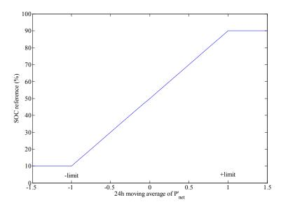
**Figure 16.** Variation of *refSOC* with the moving average of  $P'_{\text{net}}$ .
