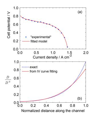
A similar procedure has been employed to reconstruct the shape of the exchange current density from the polarization data. Eighteen equidistant points belonging to the "aged" (red) polarization curve in
