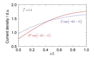
Doubling of the apparent Tafel slope could also be caused by lowering of the CCL proton conductivity. Though this effect is not considered here, it can be understood using the following arguments. The dimensionless reaction penetration depth,  $l_{\sigma}$ , for proton transport in the CCL is given by [12]:
